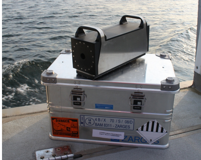
Figure F-1: Standard Bluefin Robotics 1.5 kWh Subsea Battery (From Bluefin Robotics 2013)
