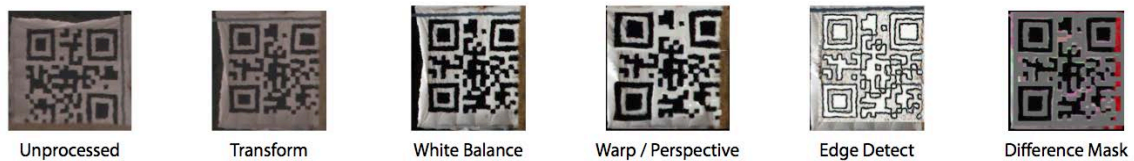
Figure 62. Process steps showing the iterative improvements of a raw captured image resulting in a readable QR code.
