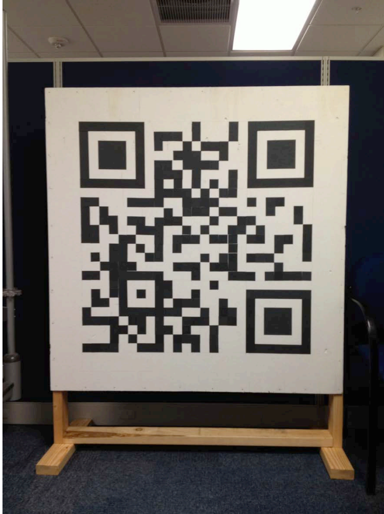
Figure 36. Field testing QR display stand constructed of basic lumber and plywood. Test QR code image: “From technical to tactical.” Version 2, ECC L(7%), 25 x 25 QR bits, 37.5 inches x 37.5 inches.
