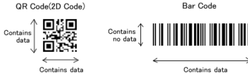
Figure 9. General characteristics of a 2D QR code compared to a 1D traditional barcode (From Sutheebanjard & Premchaiswad, 2010).
