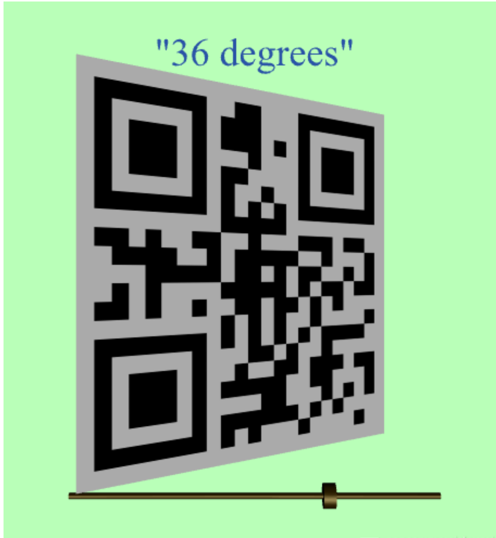
Figure 34. X3D image simulation tool displaying “http:qr.nps.edu” at an angle of 36 degrees from a perpendicular viewpoint.
