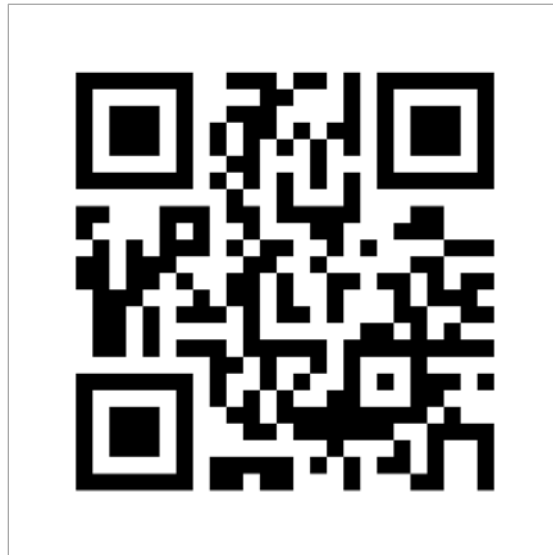
Figure 35. Test QR code image: “From technical to tactical.” Version 2, ECC L (7%), 25 x 25 QR bits. Note the necessary standards-compliant inclusion of the quiet zone 4 QR bits wide.
