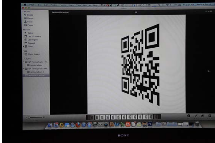
Figure 32. Capturing a digitally displayed 56 degree off-perpendicular QR code image during simulation.
