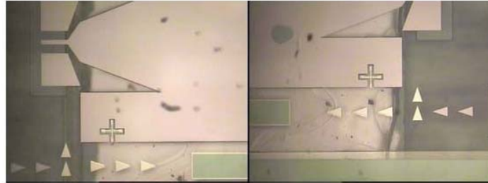
Figure IV.13 - Alignment result of bonding the top and bottom sapphire substrate layers (both layers have metallized alignment marks on the bonding side).
