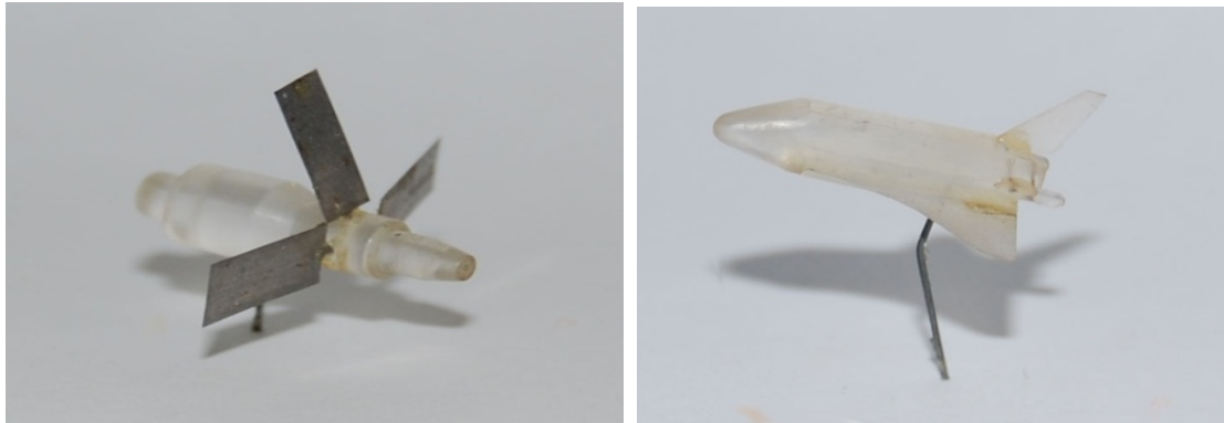
Figure 3: Long-term orbital station and Buran models studied in VU-1
