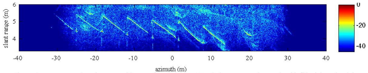
Figure 6: Reconstructed, path-corrected image of cords laid at  $10^\circ$  relative to transceiver path with fiducials at the right end of each cord and less than 0.5 m below the left end of each rope.
