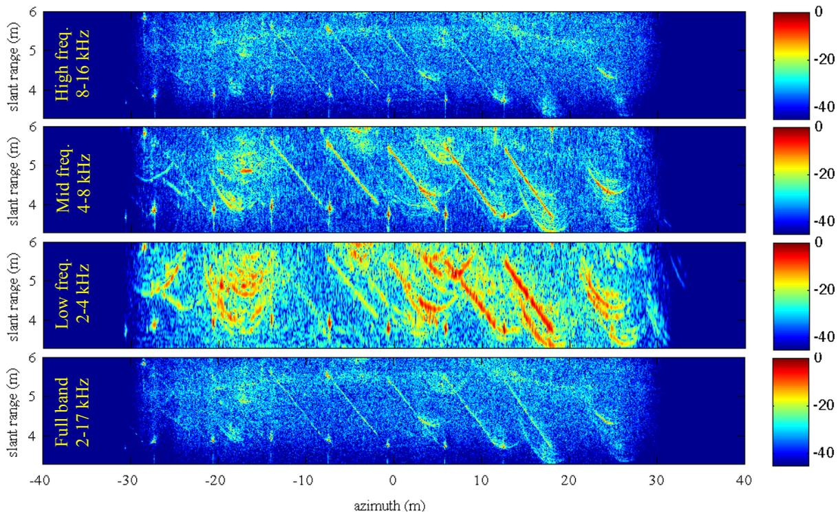
Figure 7: Reconstructed, path-corrected images of cords at  $20^\circ$  relative to transceiver path. *Bottom*: Full frequency band, 2-17 kHz, *Second from bottom*: Low frequencies, 2-4 kHz, *Second from top*: Middle frequencies, 4-8 kHz, *Top*: High frequencies, 8-16 kHz.
