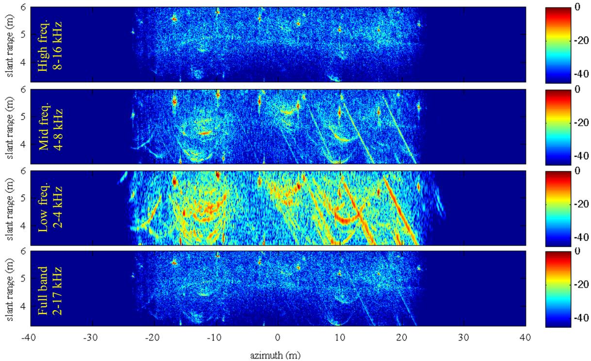
Figure 8: Reconstructed, path-corrected images of cords at  $30^\circ$  relative to transceiver path. *Bottom*: Full frequency band, 2-17 kHz, *Second from bottom*: Low frequencies, 2-4 kHz, *Second from top*: Middle frequencies, 4-8 kHz, *Top*: High frequencies, 8-16 kHz.
