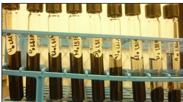
Figure 55. Showing the effect of salt addition to SWNT/SDS suspension. From left to right the salt concentration is increasing from 0 to 0.2 M NaCl
