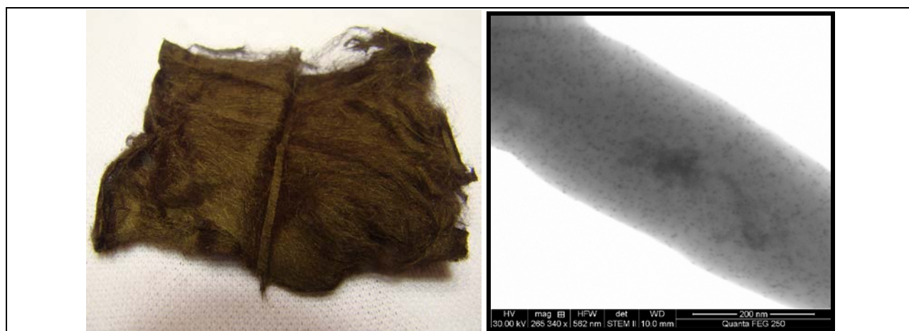
Figure 4. (A) P3HT nanofiber mat and (B) single P3HT nanofiber with PbS nanoparticles individually dispersed and distributed within the nanofiber
