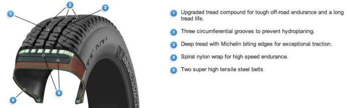
Fig. 13: Michelin LTX A/T 2 tire used for the model validation [17]
