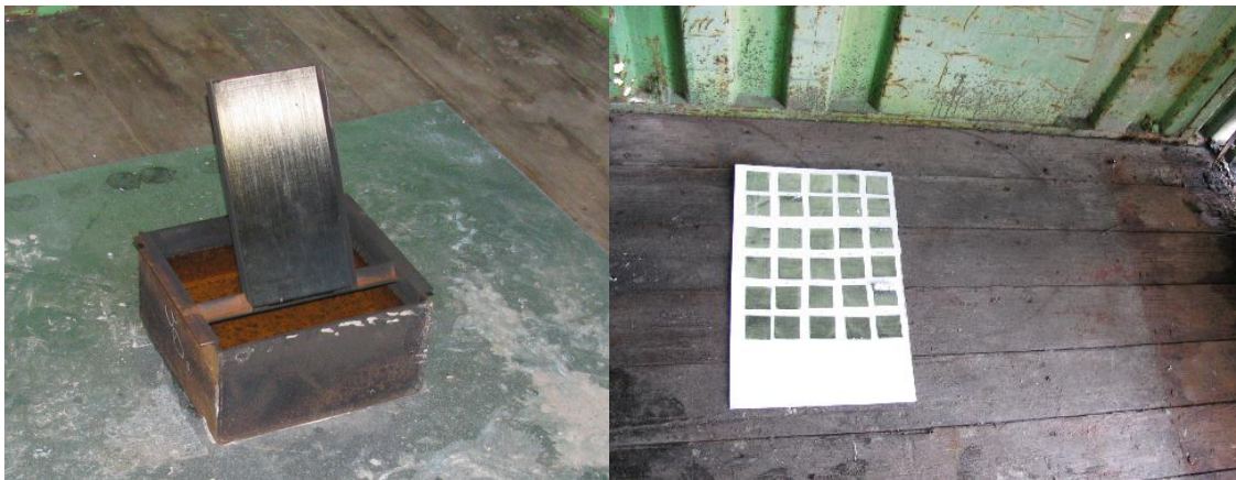
Figure 2. Composite Panel Placed in the Sample Holder (left); Array of 30 Test Coupons Placed on the Floor of the Shipping Container (right)
