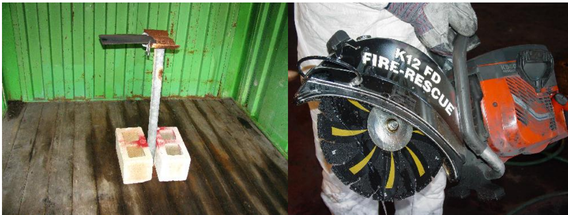
Figure 4. Composite Panel Clamped in a Support Stand (left); Husqvarna K960 Rescue Saw used to Cut Composite Panels (right)
