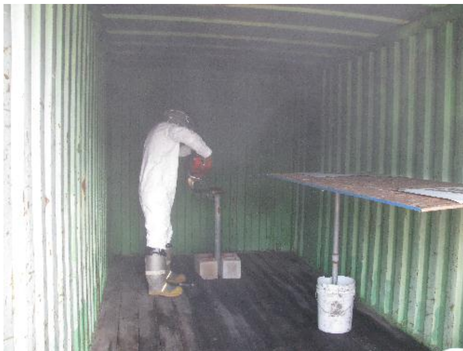
Figure 5. Composite Panel being Cut with a Rescue Saw; the Apparent Cloudiness in the Pictures is Due to the Presence of Airborne Particles Caused by the Cutting Process
