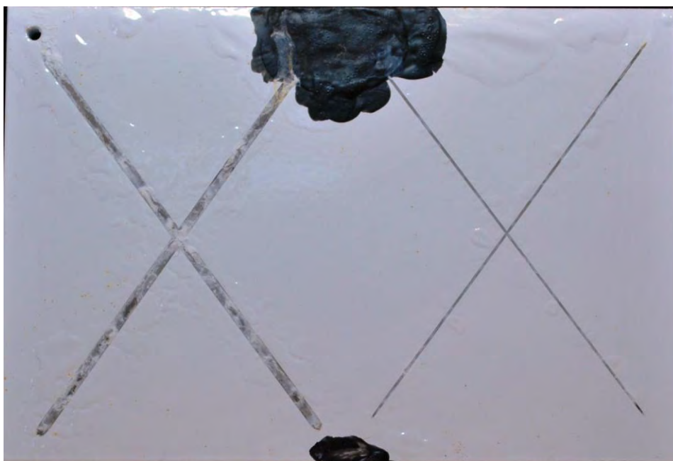
Figure 35 - UNS K91973 test panel with zinc-nickel, phosphate, pre-primer, primer, and paint protection scheme prior to test (top) and after 500 hour test (bottom) per ASTM B117. Blistering of the paint was observed near the scribes.
