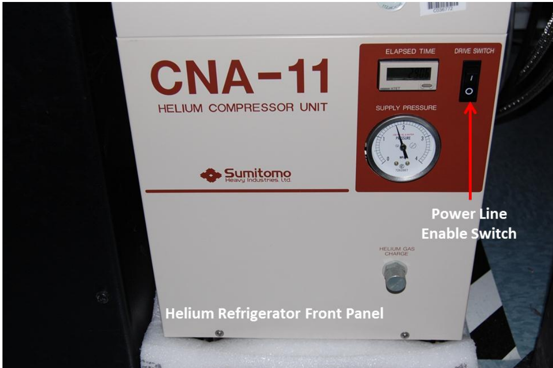
Figure 10. Helium Refrigerator Compressor Front Panel
