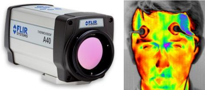
Figure 3. Infrared camera and thermal imaging data.
