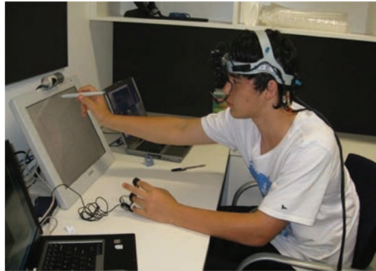
Fig. 9. Physical setup of a user completing a task using a digital pen and with GRS attached.
