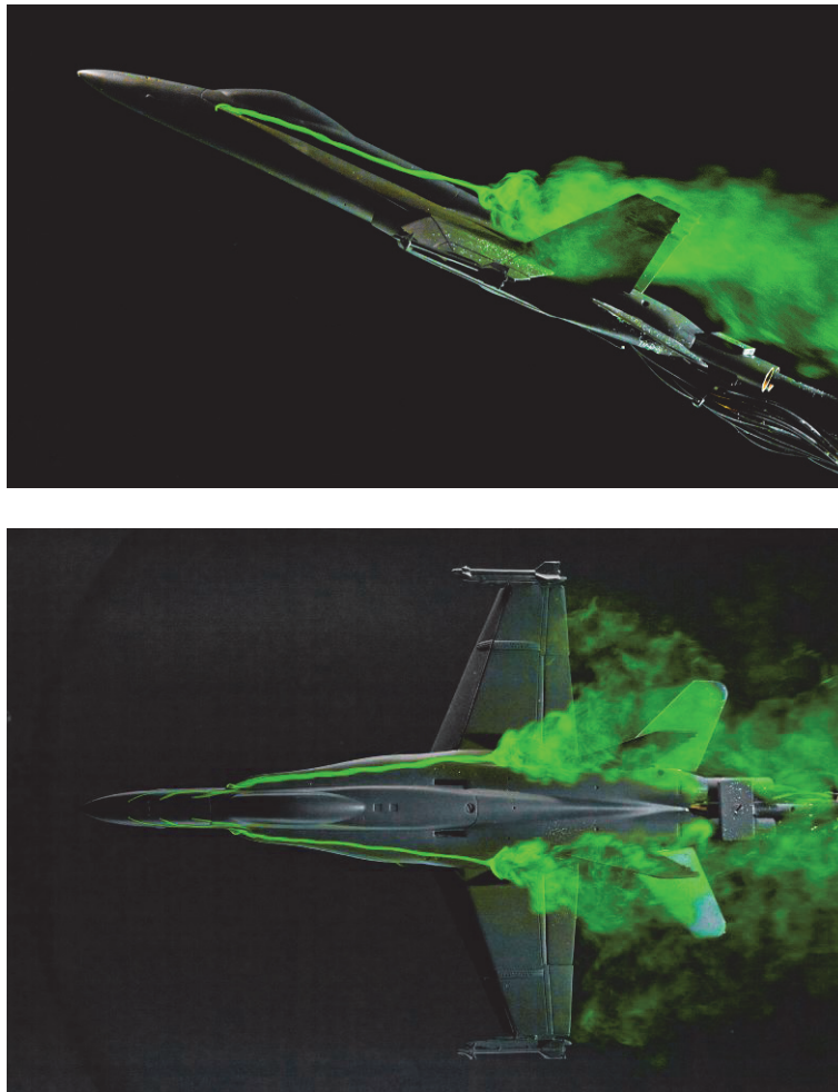
Figure 14. Side- and plan-view images of vortical flow over a 1/48 size model of an F/A-18 aircraft for \alpha = 23^\circ , as obtained in the DSTO water tunnel.
