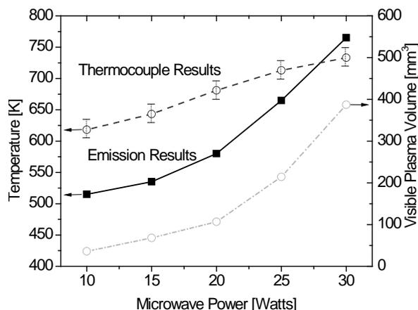
**Figure 24:** Temperature (thermocouple and rotational N<sub>2</sub> emission) of the microwave air discharge with different power levels (left Y axis); visible plasma volume with different power levels (right Y axis).
