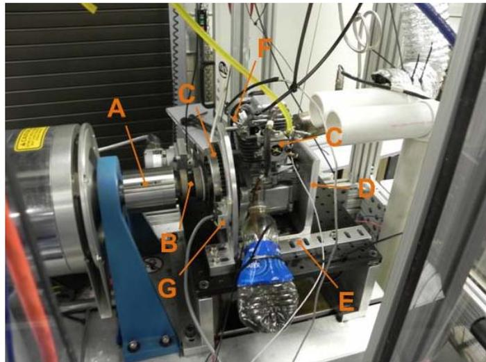
**Figure 3** Photograph of installed engine taken from intake side: **A)** dynamometer shaft adapter, **B)** coupling, **C)** flywheels, **D)** engine mounting bracket, **E)** alignment block, **F)** in-cylinder pressure sensor, **G)** ignition timing Hall Effect sensor.
