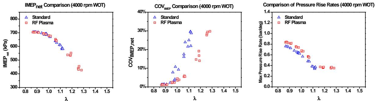
**Figure 17** Results of AFR sweep WOT at 4000 rpm
