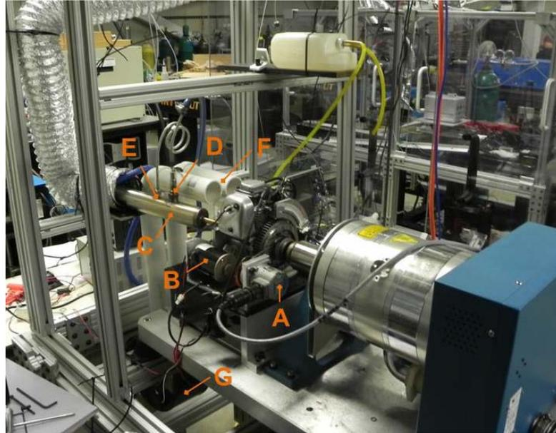
**Figure 6** Test engine viewed from the exhaust side: A) BEI encoder, B) electric starting motor, C) extended exhaust pipe, D) ECM AFR exhaust sensor, E) OTC gas analyzer probe, F) blower ducts for engine cooling.
