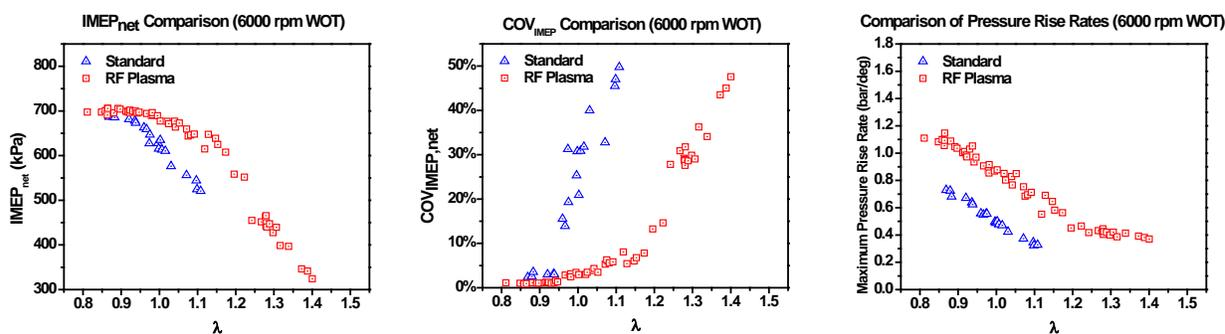
Figure 19 Results of AFR sweep WOT at 6000 rpm
