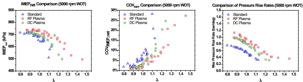
Figure 18 Results of AFR sweep WOT at 5000 rpm
