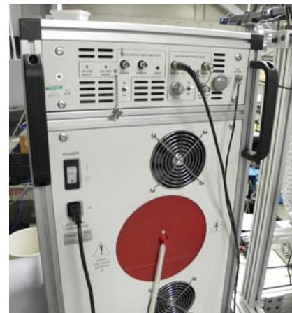
**Figure 12** High voltage radio frequency pulsar
