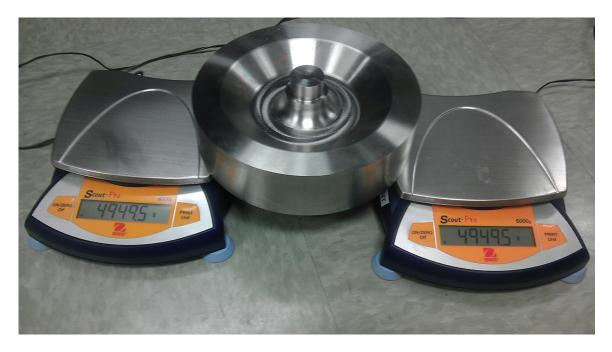
Figure 3.17: Rotor Mass Test Setup
