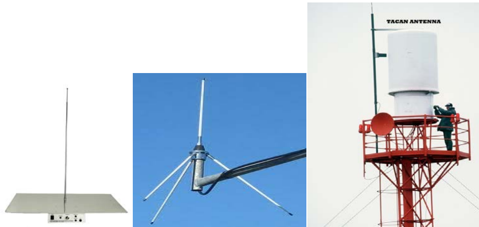
Figure G-1. Monopole Antennas
