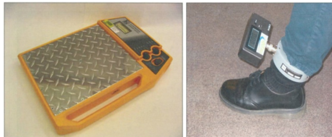
Figure 19. Induced Current Meters: a Holaday HI-3701 induced current meter and an induced current transformer HI-3702, clamped around the ankle and
