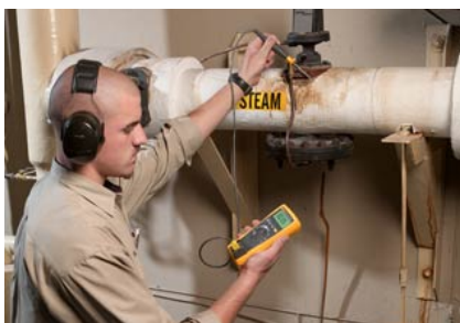
Figure 20. Contact Current Meter: Fluke 170 Multimeter being used to test for mA levels of contact current
