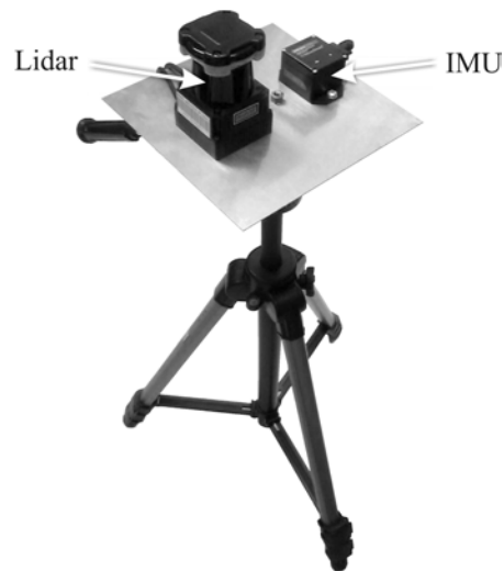
Fig. 2. Nodding device for collection of lidar data.
