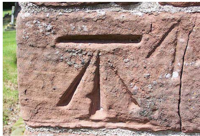
Figure 5. A Surveying ‘Bench-Mark’ in Cumbria 10
