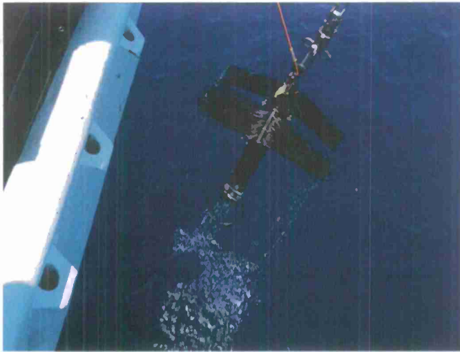
Figure 1: The Rockland VMP-500 turbulence profiler. The system is a free-falling tethered instrument package with a CTD and microstructure sensors for shear and temperature. A winch to hoist it is used from the ship's stern.
