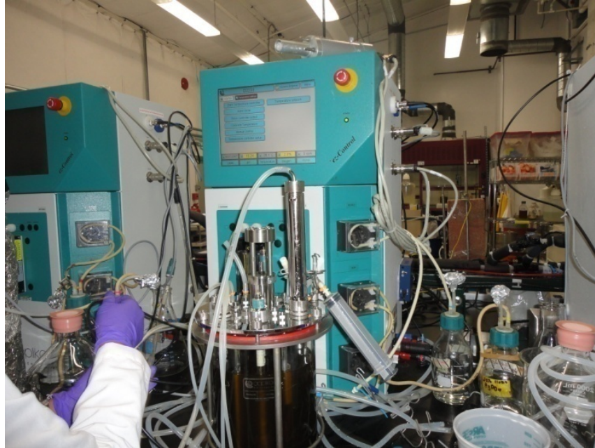
Figure 20: Bioreactor used for heterotrophic growth with beet juice as carbon source.
