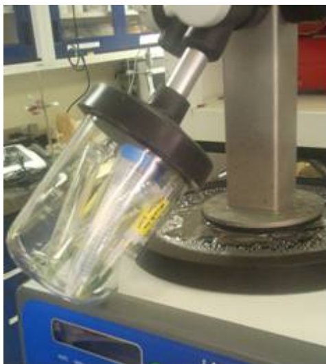
Figure 27: Freeze Dryer (left) Chlorella sp. test tubes, (right) dry Chlorella sp.
