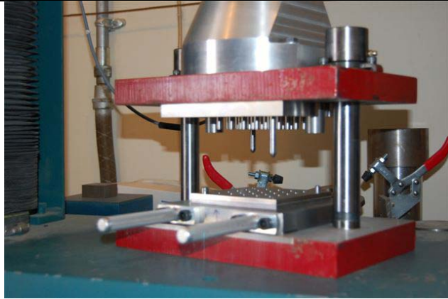
Figure 12: Die Set Placed In Press and Consolidated at 7500 psi
