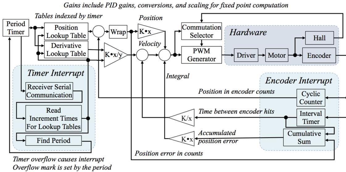
**Figure 4. Block Diagram of Stroke Position/Velocity Control**
