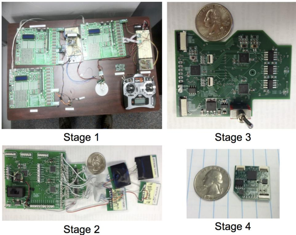
**Figure 6. Evolution of The Circuit Board Design**
