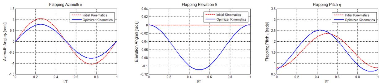
**Figure 21. Instantaneous Kinematic Motion at the Optimal and Initial Design Points**
