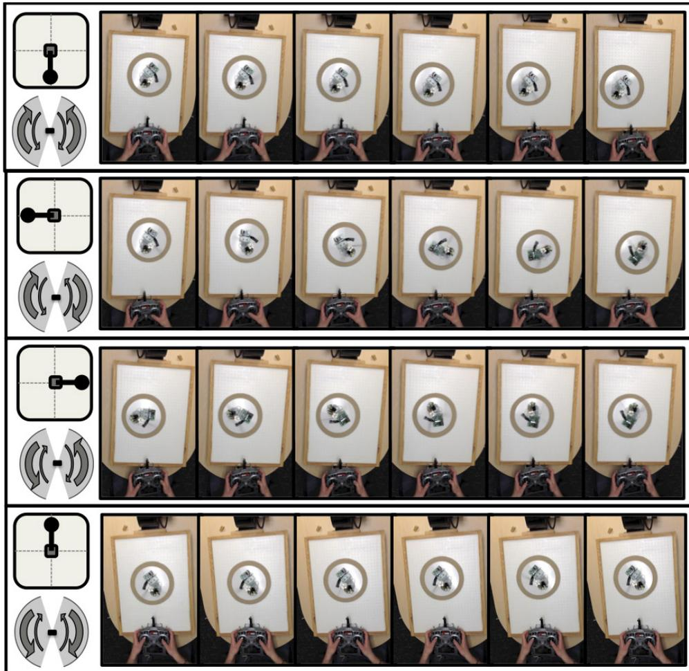
**Figure 16. Airtable Experiment, Demonstrating a Remote Controlled Prototype FWMAV Employing Split-Cycle Stroke Modulation**
