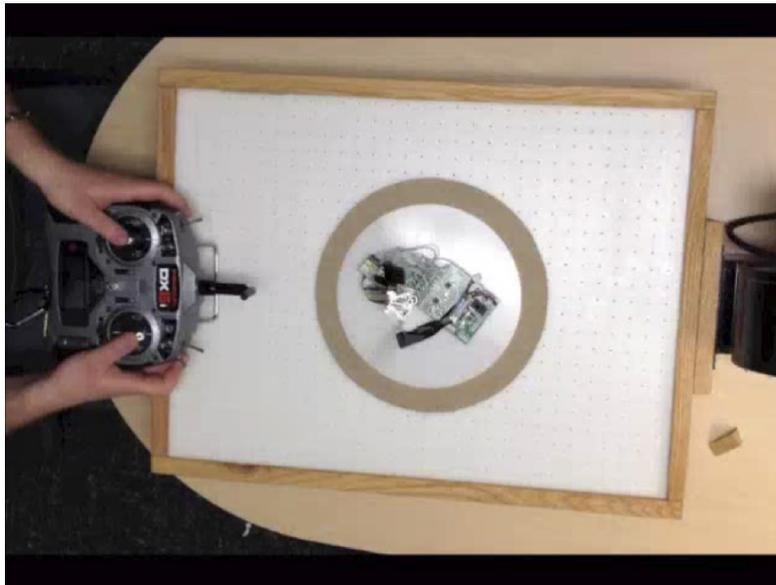
**Figure 9. The Airtable Experiment Setup with a Prototype FWMAV Mounted on a Puck**
