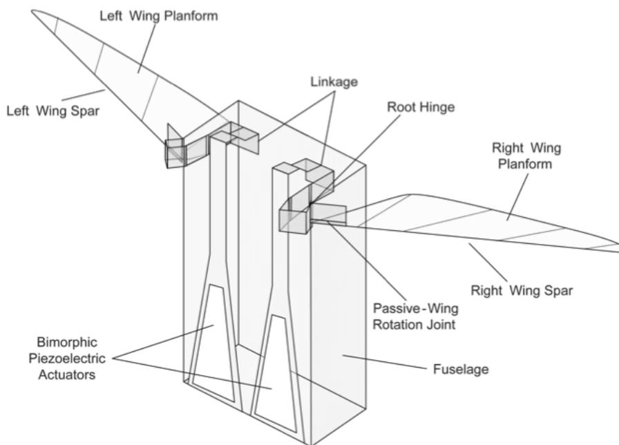
**Figure 1. General Assembly of a Minimally Actuated FWMAV**
