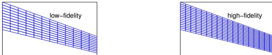
Figure 7: Low (LF) and high (HF) fidelity configurations for wing model.
