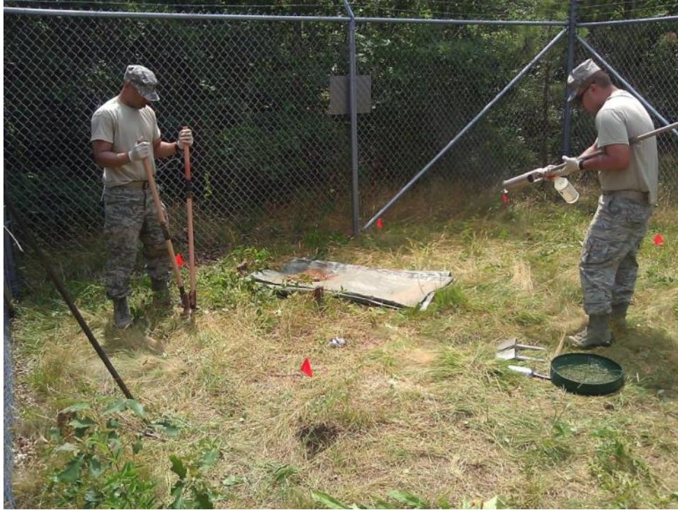
Figure 6.7. Borehole/Hand Auguring Process, Inside LF-7 Site
