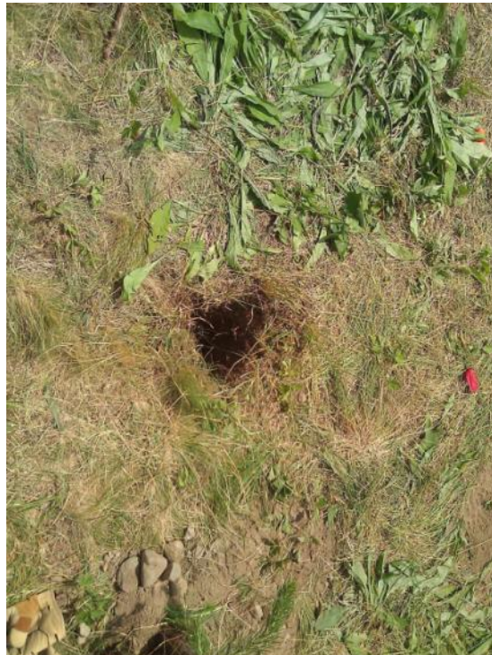
Figure 6.8. Example 2-ft-Deep Borehole, LF-7 Site
