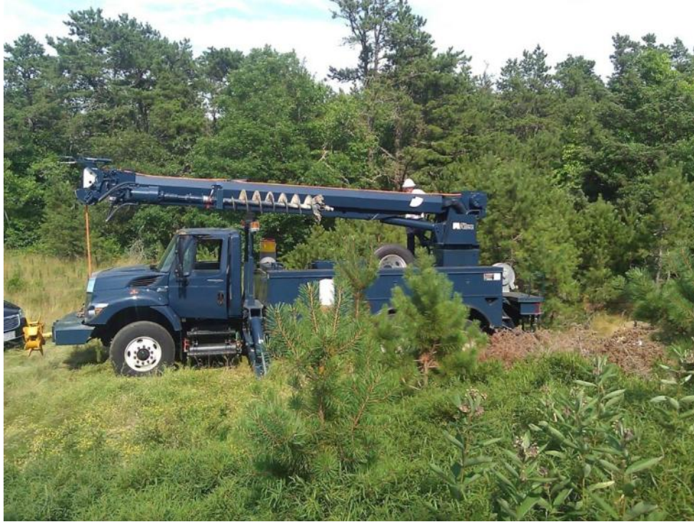
Figure 6.11. Large Auger for 6-ft Composite Samples
