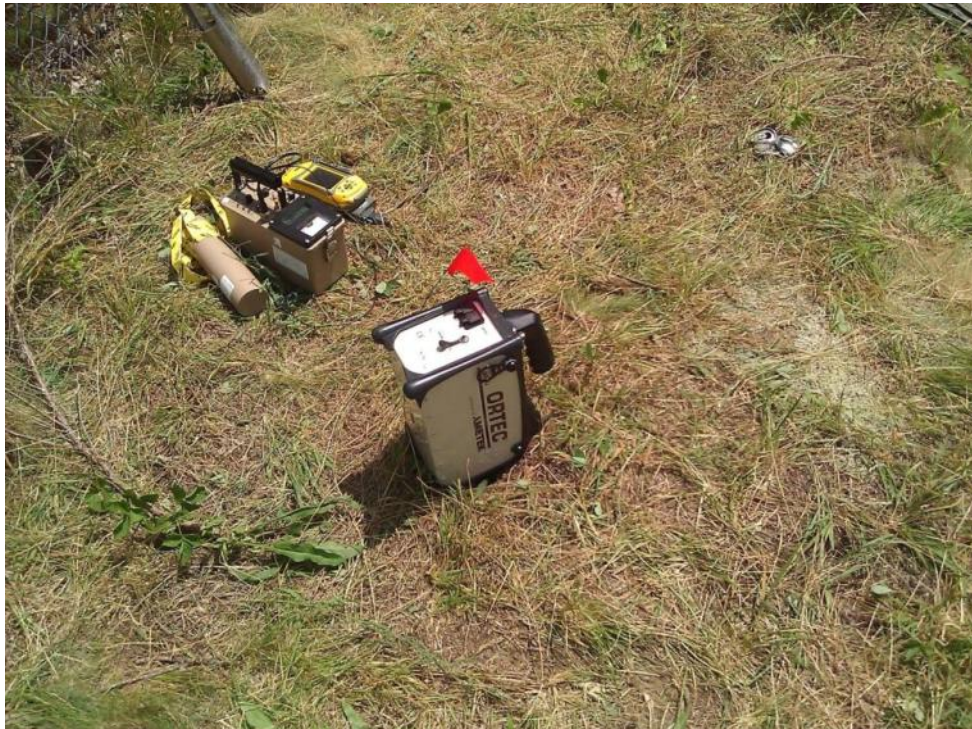
Figure 6.10. Ludlum 2221 and Ortec Detective EX, Borehole Static Measurements
