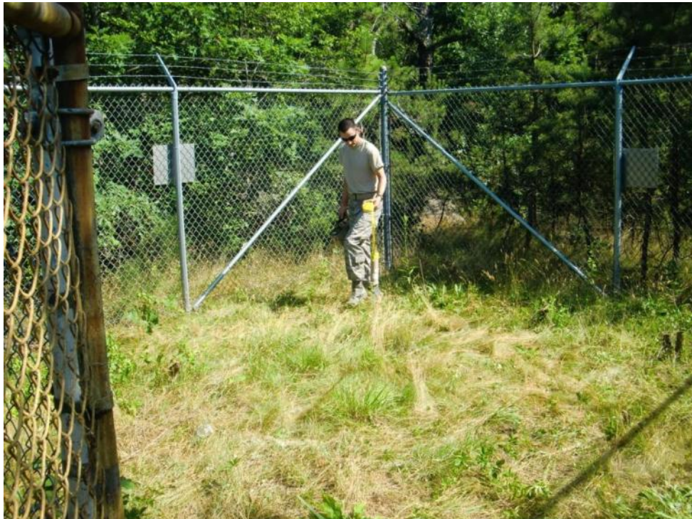
Figure 6.6. LF-7 Site, Ludlum 2221 Scan w/GPS Unit
