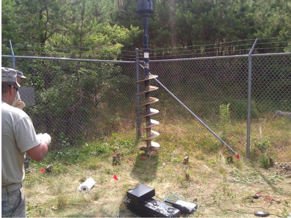
Figure 6.12b. Large Auger for 6-ft Composite Samples
