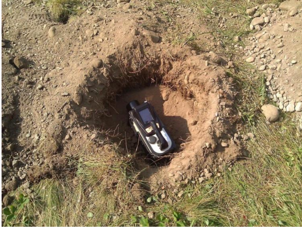
Figure 6.14. Composite Analysis Ortec Detective EX
