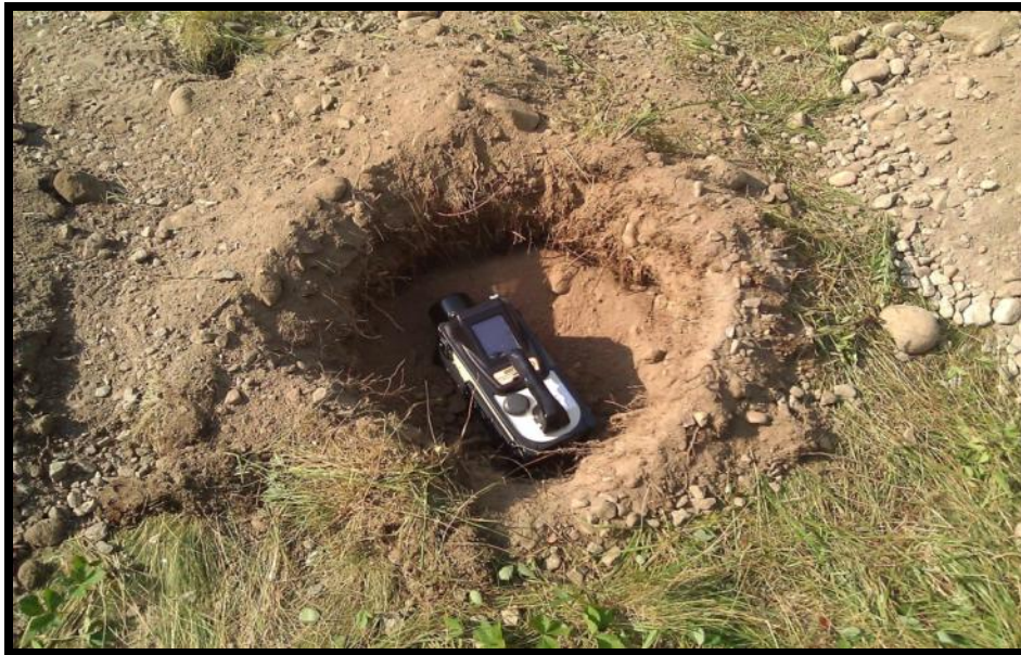
Figure 4.5. Ortec Detective EX in Borehole
