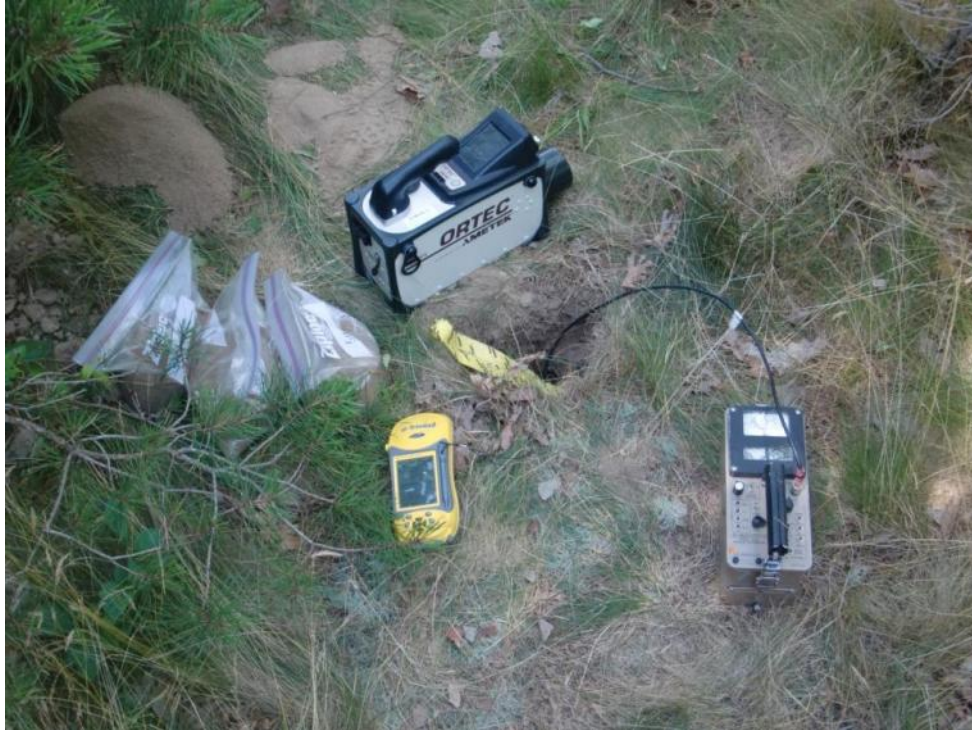
Figure 6.9. Ludlum 2221 and Ortec Detective EX, Borehole Static Measurements
