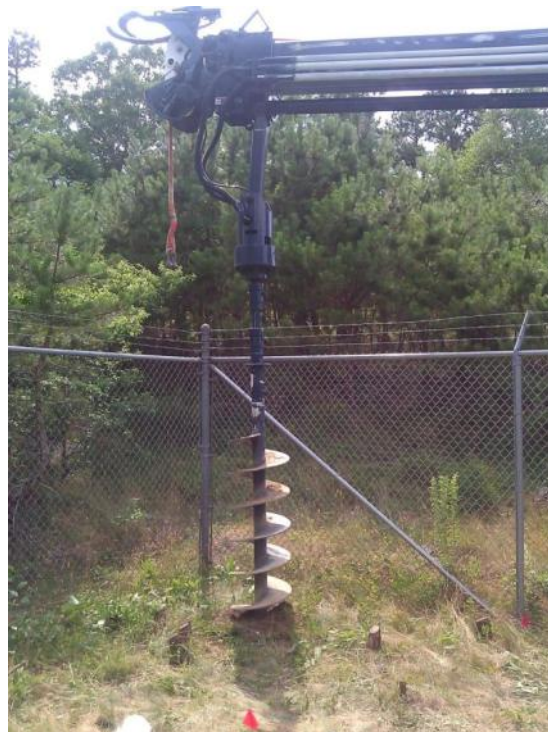
Figure 6.12a. Large Auger for 6-ft Composite Samples
