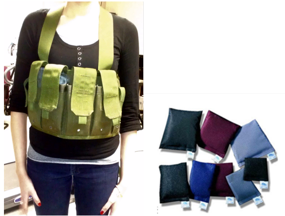
Figure 17. Simulated Bomb Vest. A 6-pocket vest was used to simulate an improvised explosive device (IED). Lead weights (top right) were inserted into the pockets to imitate the real weight of a suicide weight. The vest is worn over the head and situated on the abdominal area.
