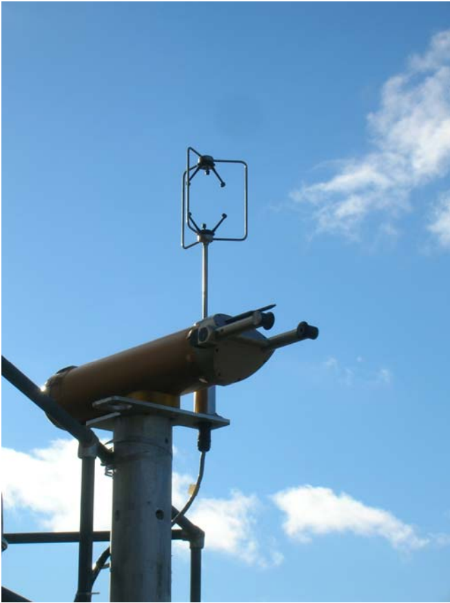
Figure 3. The cloud imaging probe and its associated sonic anemometer/thermometer deployed on the foghorn platform on Mt. Desert Rock.
