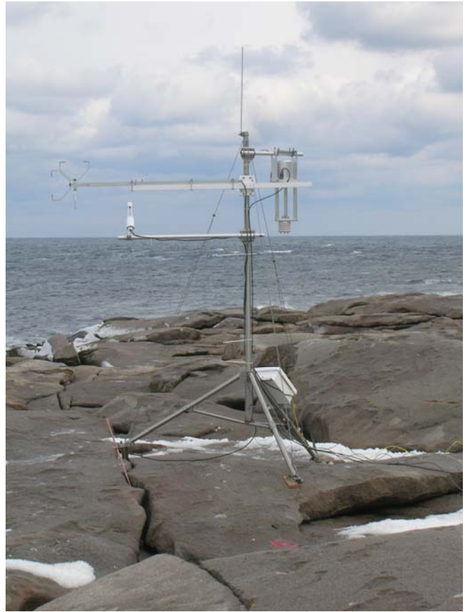
Figure 4. The “turbulence” tripod with its sonic anemometer/thermometer, carbon dioxide and water vapor sensor, and hygrometer/thermometer deployed near the shore of Mt. Desert Rock.
