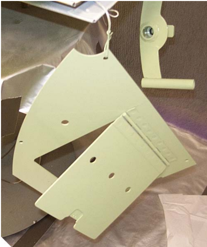
Figure 5.32: Interior Components after Application of Single-Coat, Sea-Foam Green Epoxy CARC – August 2003
