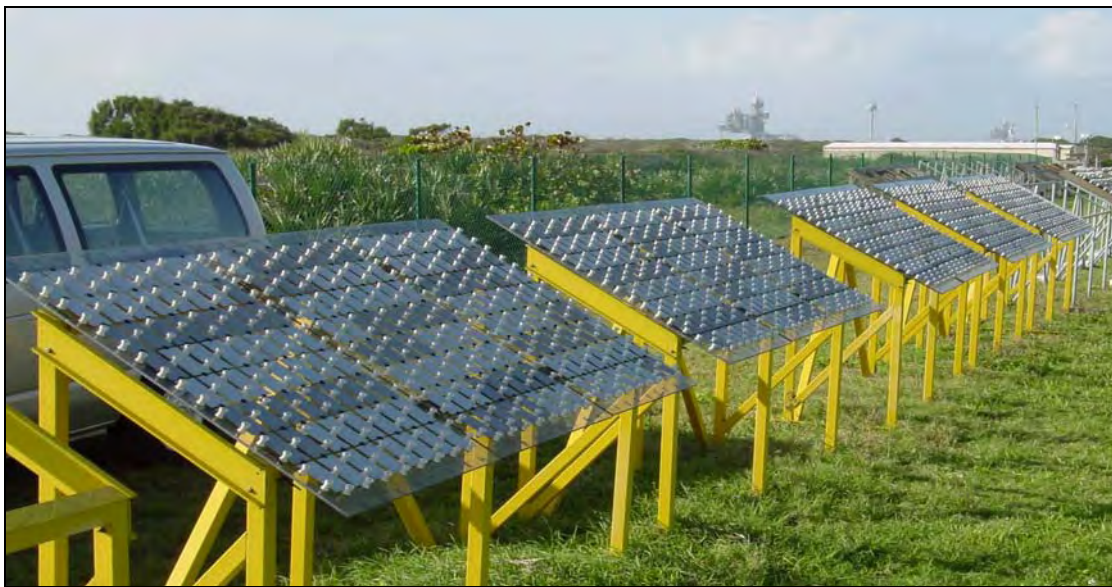
Figure 5.9.1.2: Coupon Exposure Racks
