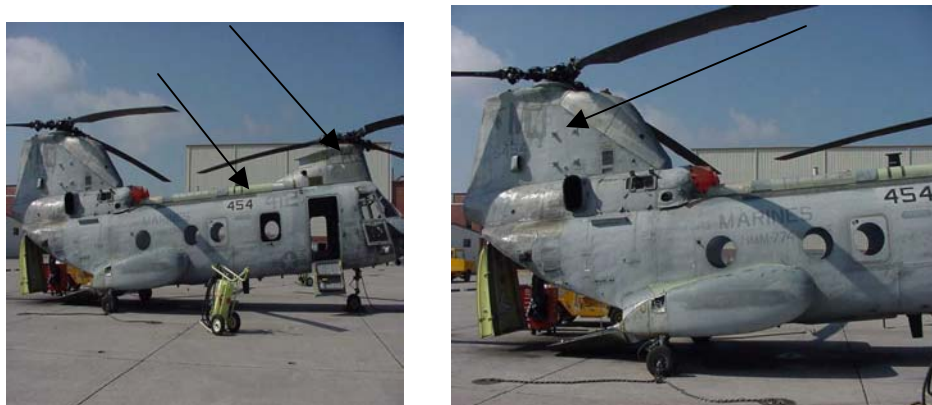
Figure 4.12: H-46 Components with TCP – NADEP CP, October 2000
