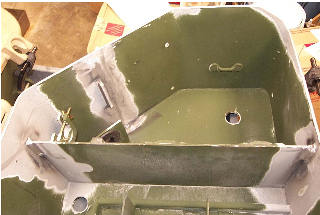
Figure 5.33: Re-Man Components – As received – November 2003 (Top) And after Grinding/Preparation of Selected Re-Work Areas (Bottom)
