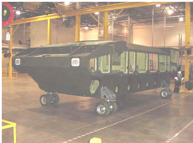
Figure 7.6.1: Spray Applied Alodine 5700 to AAAV
