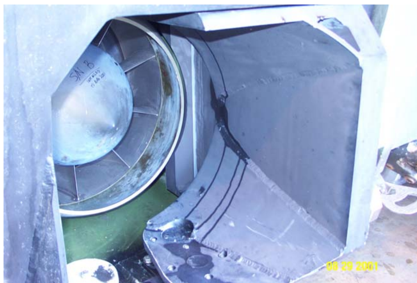
Figure 5.14: Inside of Starboard Steering Bucket after 2 Weeks in Service
