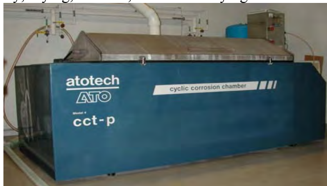
Figure 5.7.2.1: Test Chamber Configuration Used for GM 9540P
