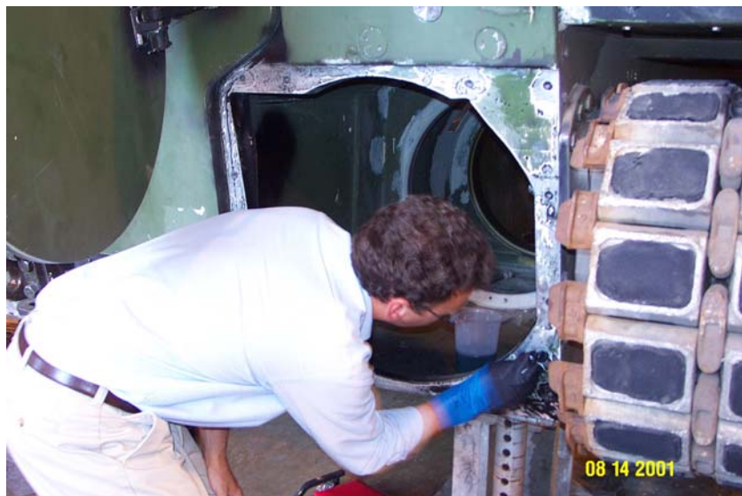
Figure 5.11: Application of TCP Coating on Seal Plate Mating Surface
