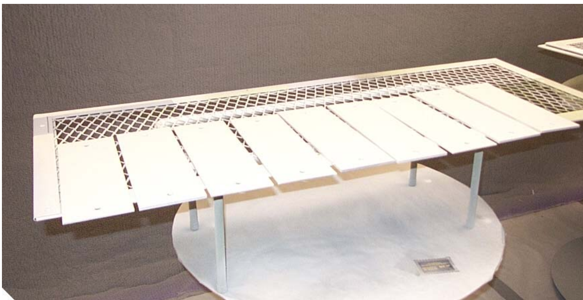
Figure 5.35: QC panels after MIL-P-53022 Primer Application
