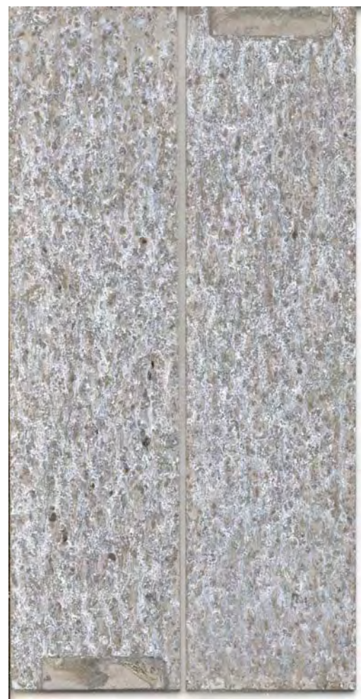
Figure 5.1.2.1: Alodine 5200 on 2024 and 2219 After 1 Week Exposure
