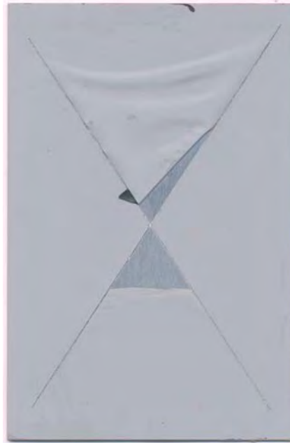
Figure 5.5.2.8: Severe Delamination of Oxsilan AL 0-500 Pretreated on Al 7075 Coated With 85582C2/25285 Coating System at 1 Week Exposure
