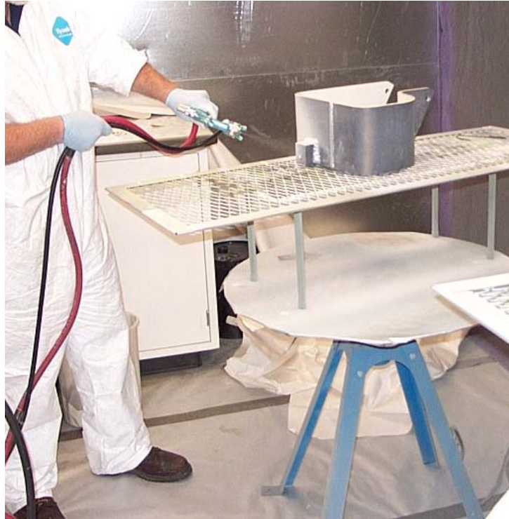
Figure 5.31: Primer Application – Left Headlight Guard – August 2003
