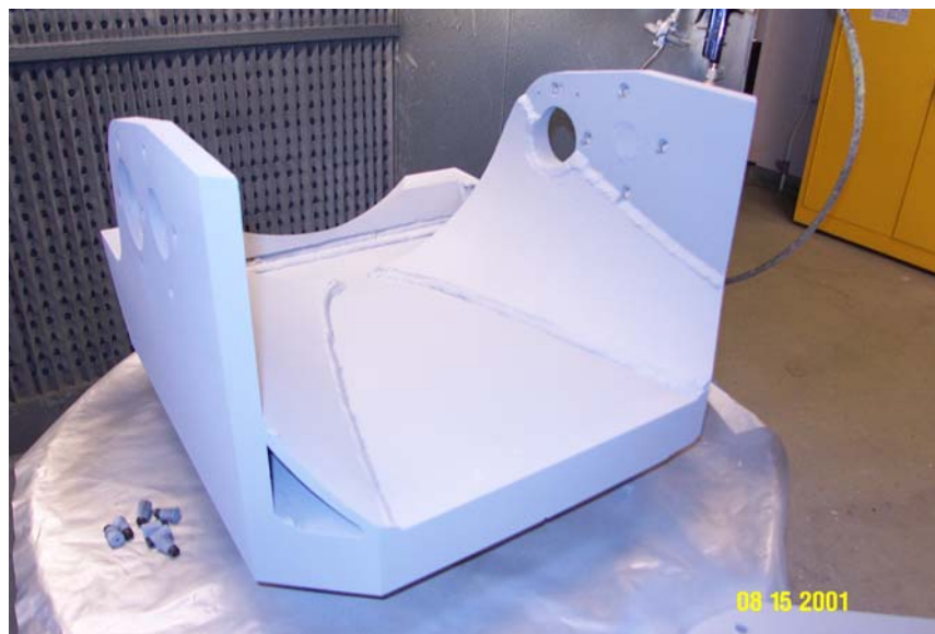
Figure 5.9: Steering Bucket after Topcoat Application with MIL-C-53039
