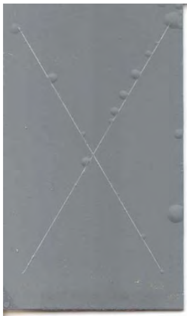
Figure 5.6.3.5: Pretreatments With 85582 NC/85285 Coating System on Al 2219 after 500 Hour Exposure
