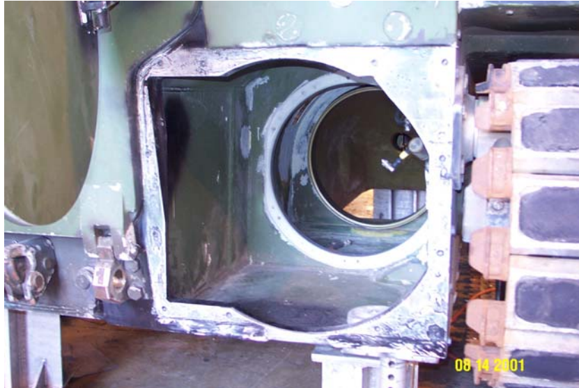
Figure 5.10: Seal Plate Mating Surface after Corrosion Removal
