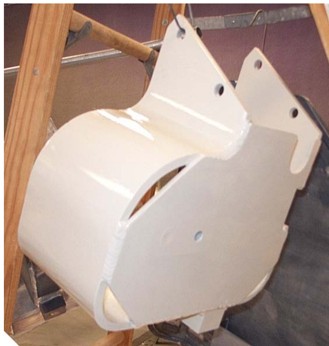
Figure 5.31: Primer Application – Left Headlight Guard – August 2003
