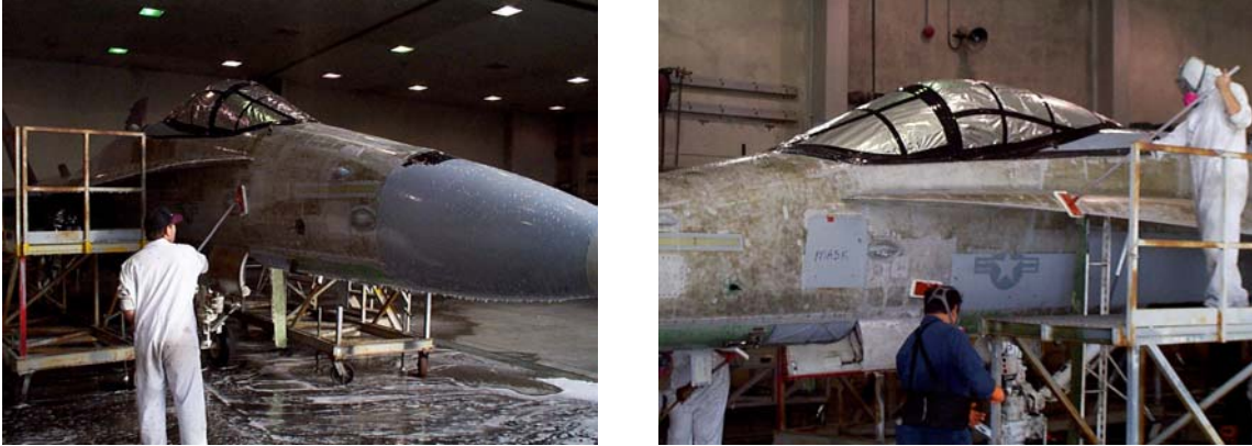
Figure 4.7: TCP Application on BUNO 163757, North Island, November 2000
