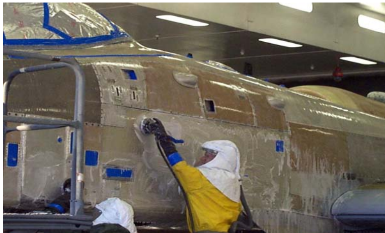
Figure 4.1: Application of PreKote at Hill AFB
