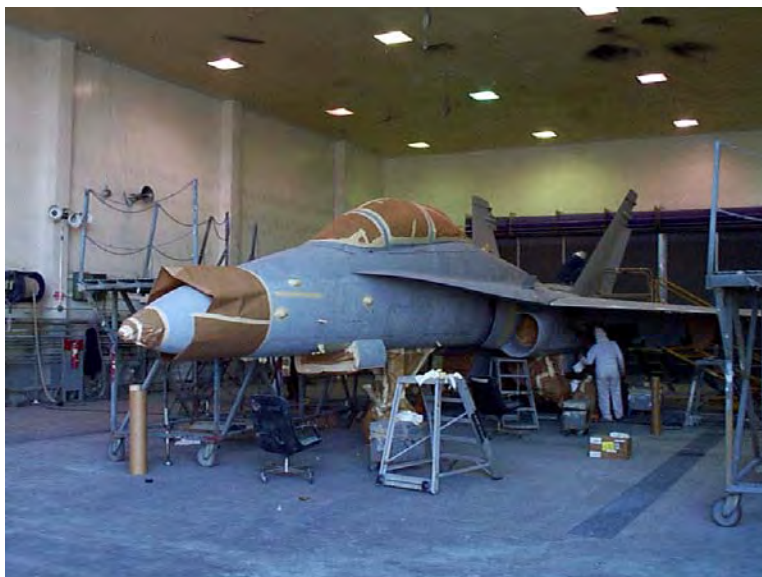
Figure 7.5.1: F/A-18 after TCP Application and Painting
