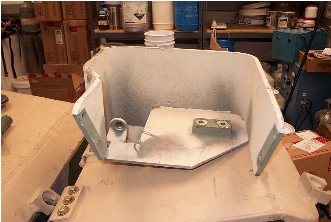
Figure 5.33: Re-Man Components – As received – November 2003 (Top) And after Grinding/Preparation of Selected Re-Work Areas (Bottom)
