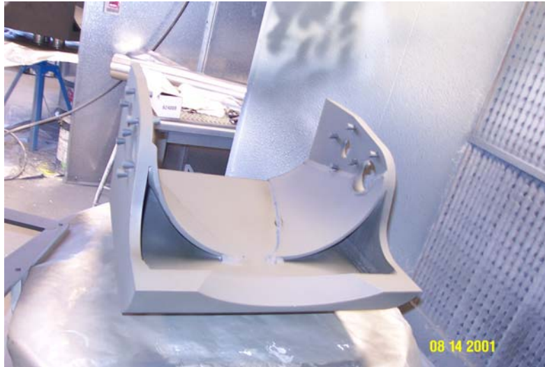
Figure 5.8: Steering Bucket after Priming with MIL-PRF-85582 NC
