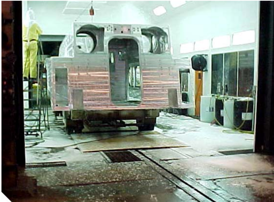
Figure 5.15: EFV E3 Spray Processing – LATP
