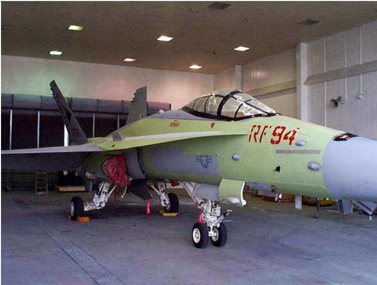
Figure 4.9: F/A-18C with TCP after Primer Application – November 2000, NORIS
