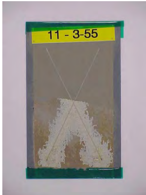
Figure 5.8.2.5: Sanchem 7000 with 53030 Primer, Rating: 0
