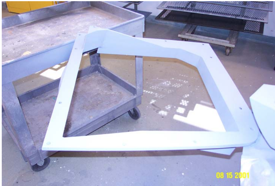
Figure 5.10: Seal Plate after Topcoat Application with MIL-C-53039
