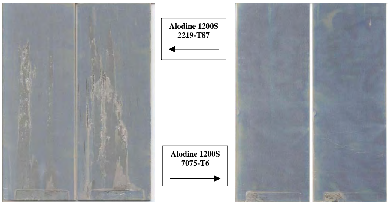
Figure 5.1.2.7: Alodine 1200S on 2219 and 7075 After 2 Weeks Exposure
