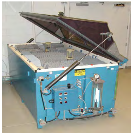
Figure 5.5.2.1: Test Chamber and Panels Used for ASTM B 117
