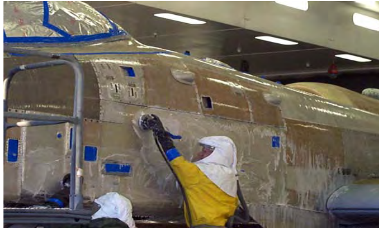
Figure 7.3.1: Application of X-It PreKote
