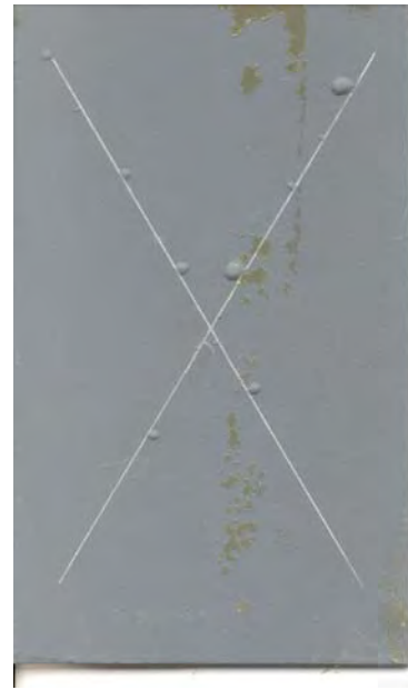
Figure 5.6.3.5: Pretreatments With 85582 NC/85285 Coating System on Al 2219 after 500 Hour Exposure
