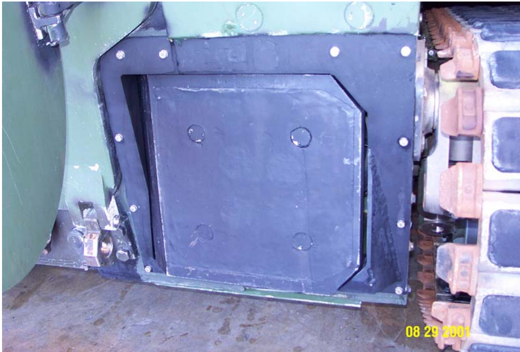
Figure 5.13: Starboard Steering Bucket and Seal Plate after 2 Weeks in Service
