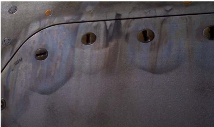
Figure 4.8: Iridescent Blue Coloration of As-deposited TCP
