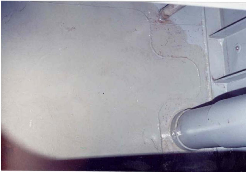
Figure 5.1: LCAC-26 Oily Waste Tank with TCP Test Patch
