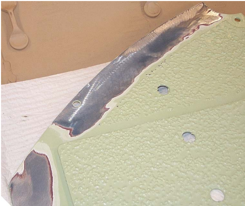
Figure 5.34: Re-Man Parts after Pretreatment of Selected Test Areas (Top) And after Primer and Top-Coat Application (Bottom)
