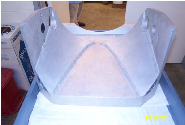
Figure 5.7: TCP Coating after Drying
