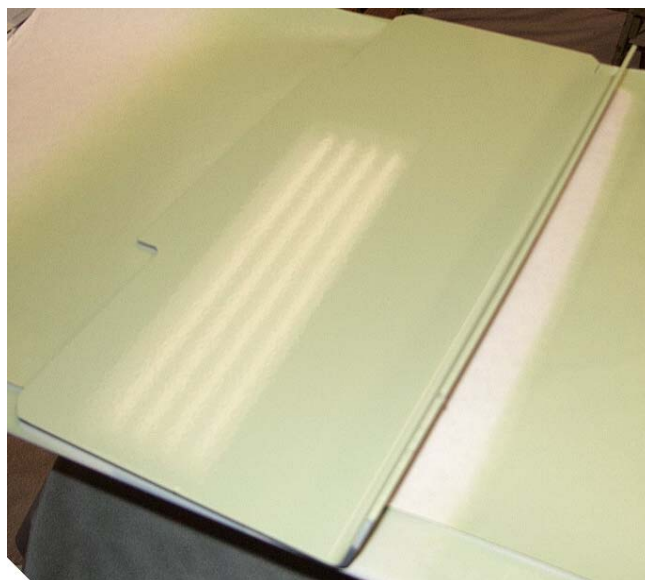
Figure 5.32: Interior Components after Application of Single-Coat, Sea-Foam Green Epoxy CARC – August 2003
