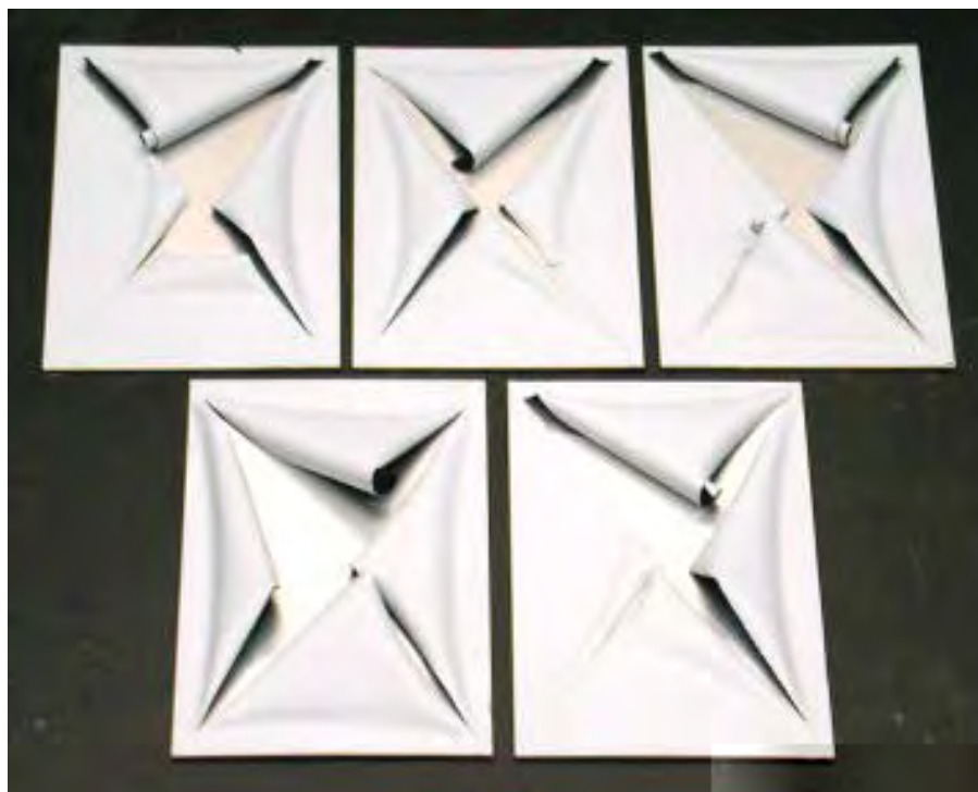
Figure 5.5.2.9: Severe Delamination of Oxsilan AL 0-500 Pretreated on Al 7075 Panels with 85582C2/25285 Coating System at 2 Weeks Exposure
