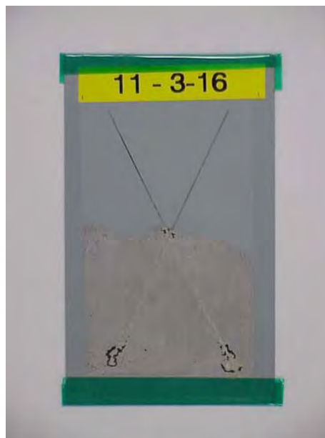
Figure 5.8.2.2: TCP with 23377 Primer, Rating: 82
