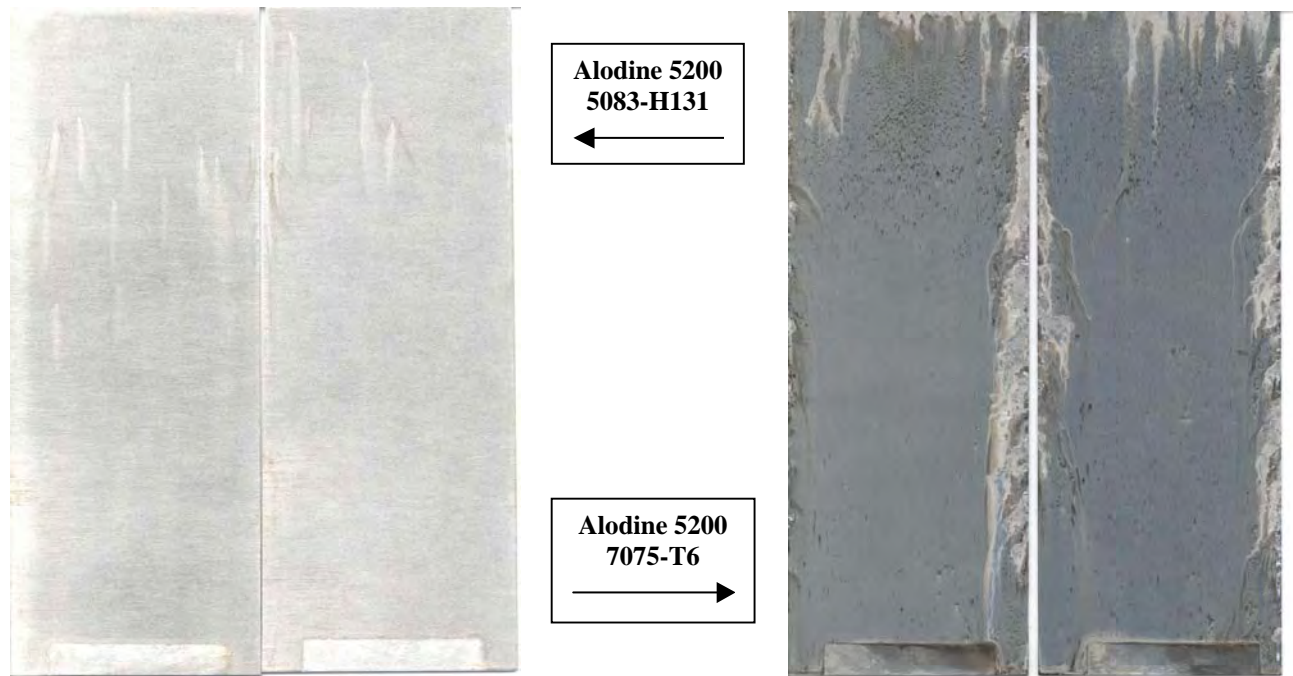
Figure 5.1.2.2: Alodine 5200 on 5083 and 7075 After 1 Week Exposure
