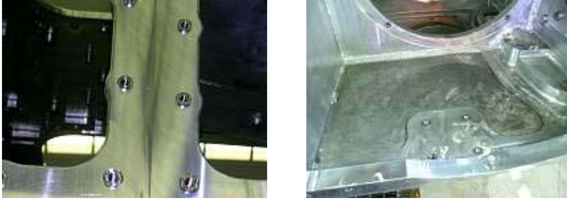
Figure 5.16: Minimal TCP Color Change Observed Near Inserts
