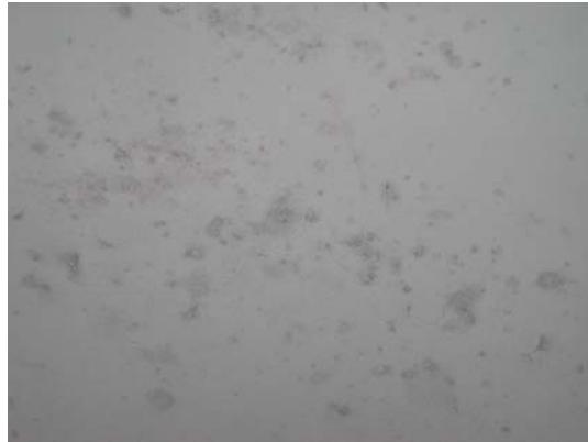
Figure 4.5. Open Area Corrosion
