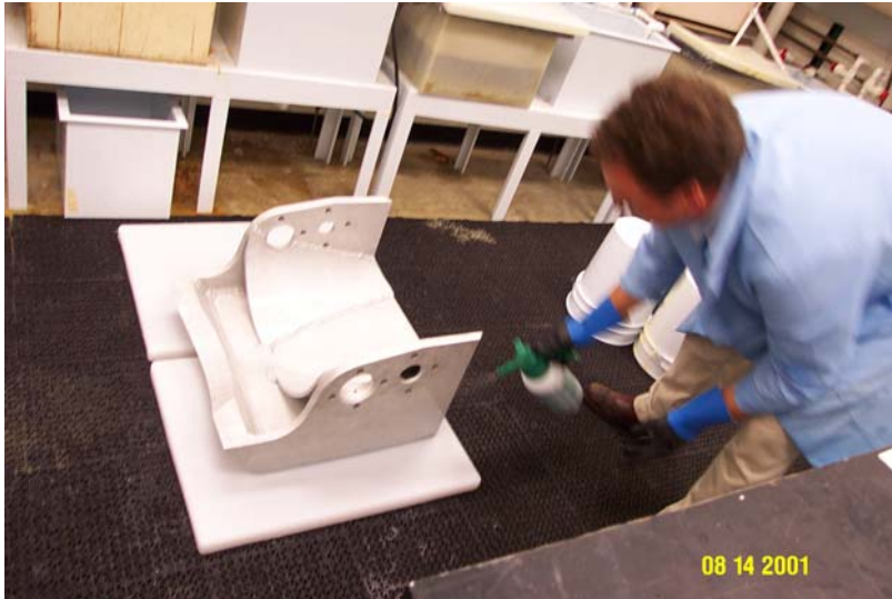
Figure 5.6: Application of TCP
