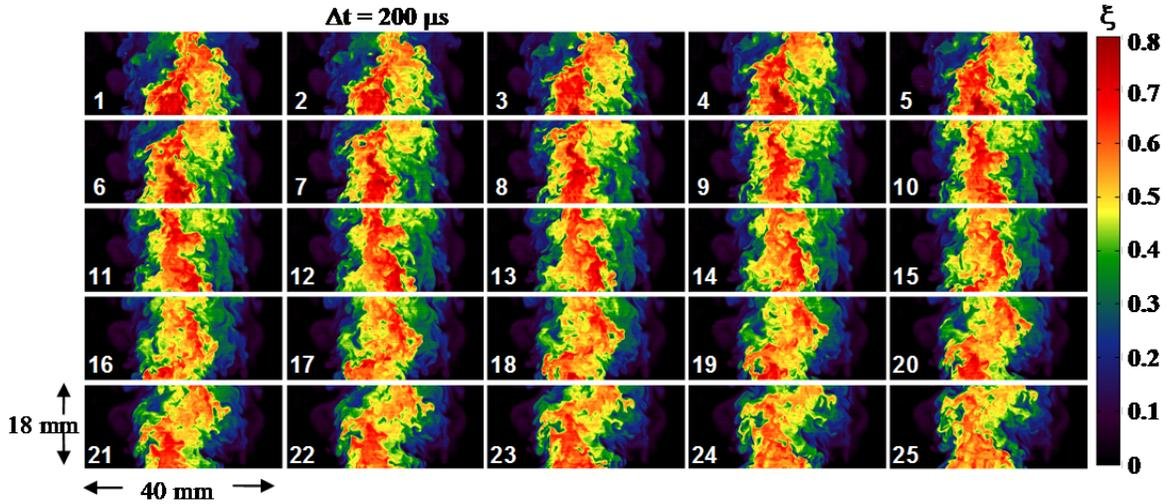
Fig. 2 – 25-frame (of 100), 5-kHz sequence of the mixture fraction field in a turbulent ( $Re = 15000$ ) non-reacting propane jet issuing into air. Image sequences are shown for an axial position of  $x/d = 10$ . The images were acquired at 10 kHz, but only every other image ( $200 \mu s$  spacing) is shown for clarity. The total time represented is 5 ms.
