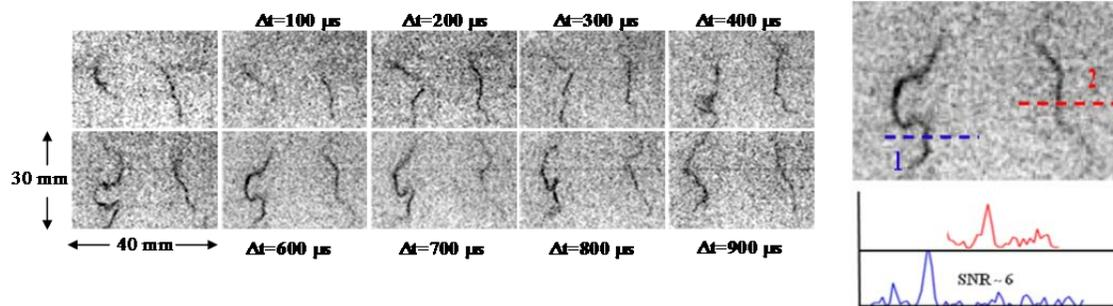
Fig. 10 – A ten-frame CH PLIF image sequence in DLR Flame A at an axial position of 175 mm downstream of burner exit. The spacing between the images is 100  $\mu\text{s}$ , corresponding to a 10-kHz acquisition rate.
