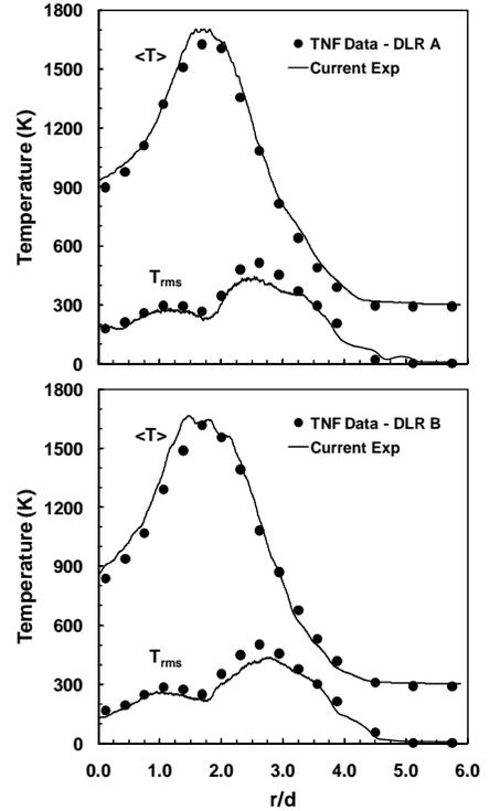
**Fig. 7 – Comparisons of the time-averaged mean and RMS radial temperature profiles measured at an axial position of  $x/d = 20$  in the DLR flames from current high-speed imaging (solid line) and the reference point data (symbols) from Sandia National Laboratories [20]. (Top) DLR flame A; (Bottom) DLR flame B.**
