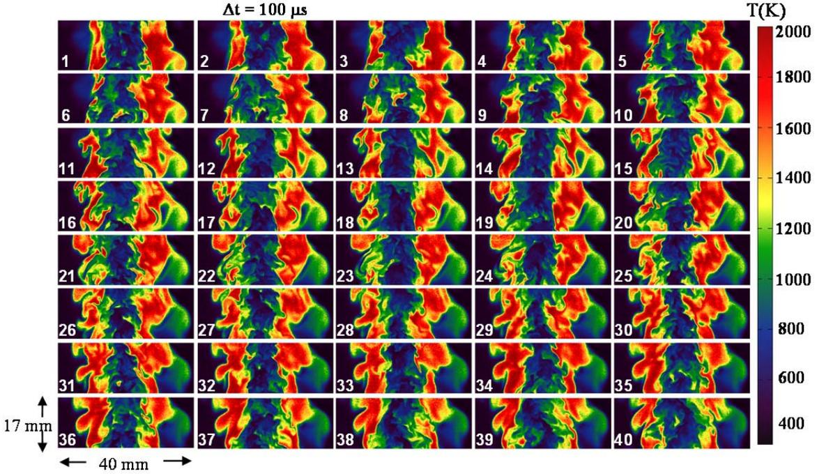
**Fig. 5** – 40-frame (of 100), 10-kHz sequence of the temperature field in a turbulent ( $Re = 22800$ ) non-premixed jet-flame issuing into air. Fuel mixture is 22.1% CH<sub>4</sub> /33.2% H<sub>2</sub> / 44.7% N<sub>2</sub> and  $Re = 22,800$  (DLR B Flame). Image sequences are shown for an axial position of  $x/d = 10$ . The total time represented is 4 ms.
