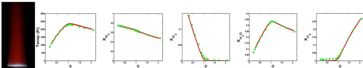
**Fig. 9** – (Left) Photograph of a near-adiabatic premixed  $\text{H}_2$ -air flame. (Right) Measurements (green symbols) of temperature and major species as compared to equilibrium calculations (red lines).
