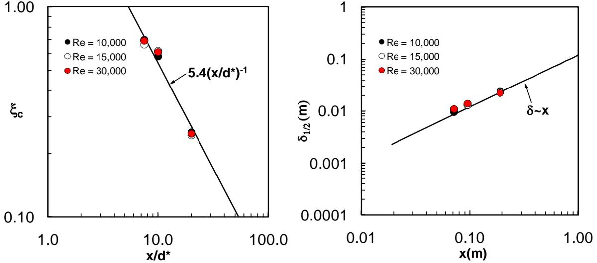
**Fig. 3 – Comparison between measured mean centerline mixture fraction,  $\xi_c$  and mixture fraction scaling laws for a turbulent jet. (b) Comparison between measured jet-half-width ( $\delta$ ) and scaling laws for a turbulent jet. Note, three Reynolds number conditions are reported at each axial position.**
