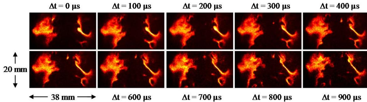
**Fig. 11: 10-kHz sequence of the  $\text{CH}_2\text{O}$  field in a turbulent non-premixed  $\text{CH}_4$  flame ( $\text{Re} = 6000$ ). Images are centered at  $x/d = 8$ .**
