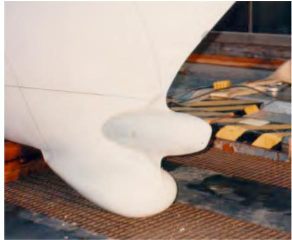
Fig. 4. Retrofit bow bulb on DDG 51 model
