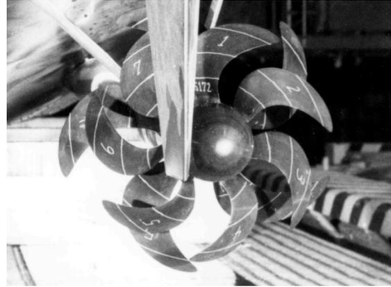
Fig. 2. DDG 51 CR-1 design model propellers
