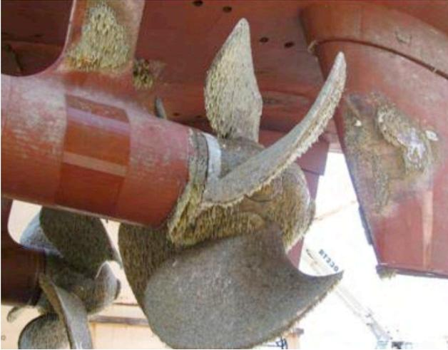
**Fig. 15.** Severe biofouling on STOCKDALE (DDG 106)
