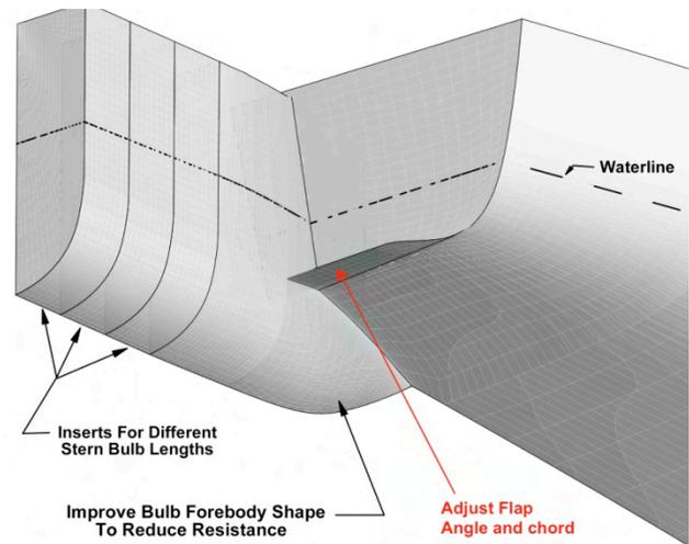
**Fig. 9.** Stern end bulb Phase III design iterations
