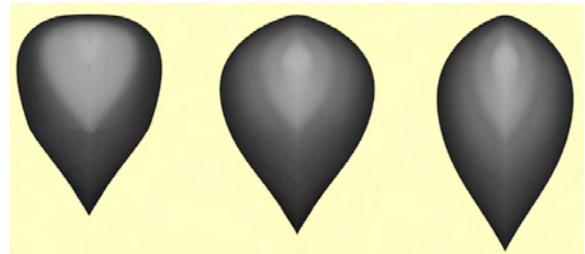
Fig. 5. Cross-section shapes of candidate bow bulbs
