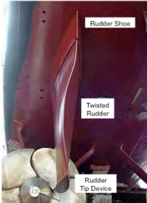
**Fig. 14.** Twisted rudder on BULKELEY (DDG 84)
