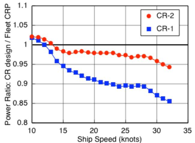
Fig. 3. DDG 51 contra-rotating propeller designs model-scale powering performance
