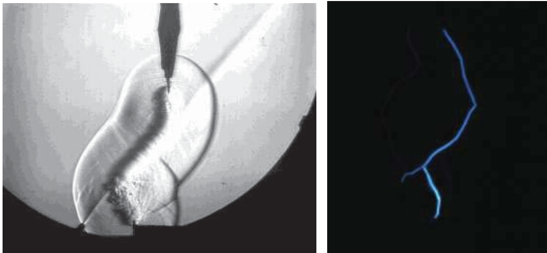
Fig.5.5.8. Schlieren image HV discharge + He jet (delay 20 \mu s) and photo of the discharge.
