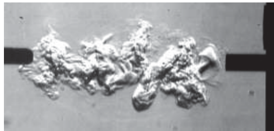
Fig.2.1.3. Typical schlieren image of post-discharge thermal distortion, t=200 \mu\text{s} .
