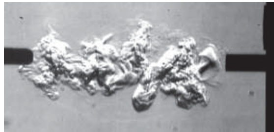
Fig.5.2.3. Typical schlieren image of post-discharge thermal distortion, t = 200 \mu\text{s} .
