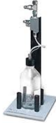
Figure 5. Photo of TSI 3076 atomizer for aerosol generation
