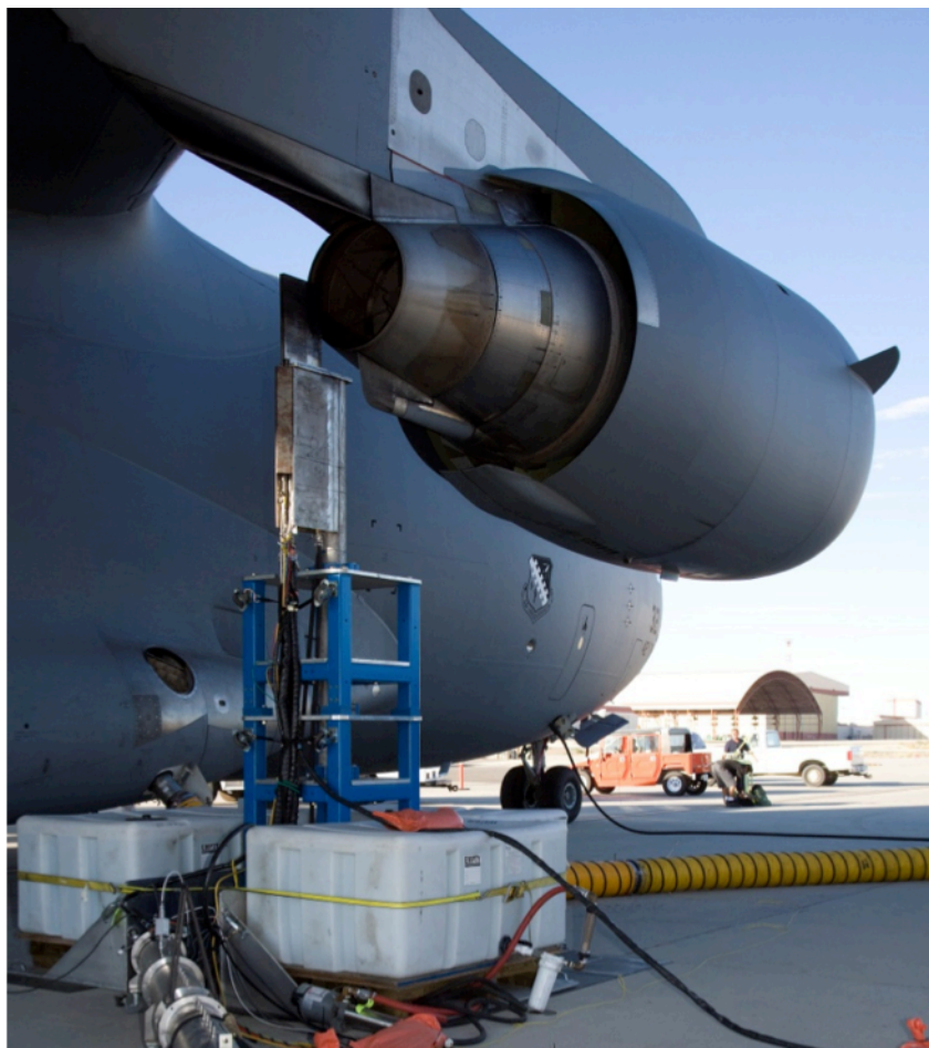
Figure 16. Photo of the sampling rake setup for C-17 emissions test. The probes are located at the top of the rake.
