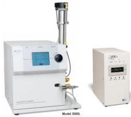
Figure 4. Photo of TSI SMPS system
