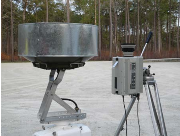
Figure 4. The thermal imager (Radiance I high-resolution thermal imaging camera) on the right and the vertically pointing radar (Furuno FR2155-BB 50 kW X-band radar with a vertically-pointing parabolic dish antenna) employed by the IVAR project to confirm targets tracked by an avian radar at night were birds.
