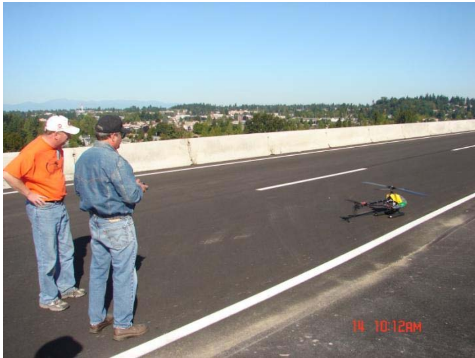
Figure 5. Remotely controlled helicopter with onboard recording GPS used to validate spatial coordinates of targets tracked by the avian radar system.
