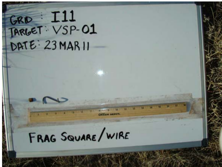
Figure 26. Image of the items found from the single location with a mV reading above the verification remediation signal threshold (channel 2 reading of 9.7).
