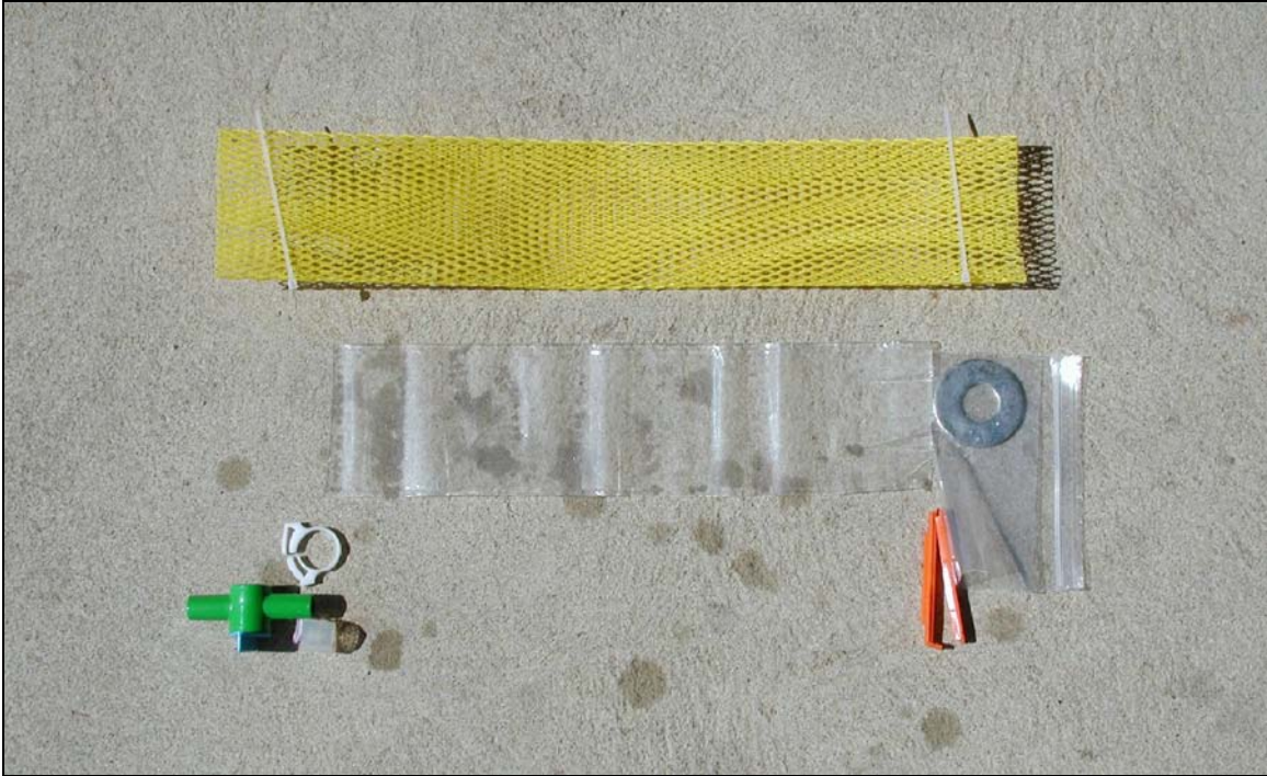
Figure 2. Disassembled regenerated cellulose dialysis membrane diffusion sampler, showing component parts.
