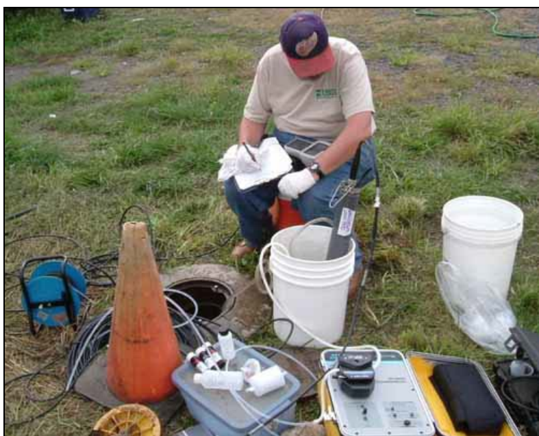
Figure 11. Low-flow purging set up for a 4-inch diameter well.
