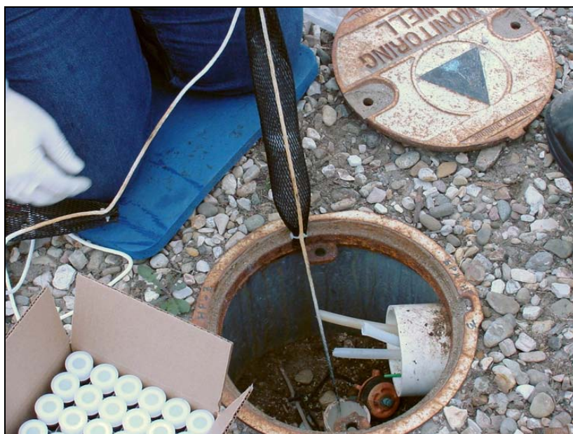
Figure 10. Removal of diffusion sampler from a well prior to sampling.
