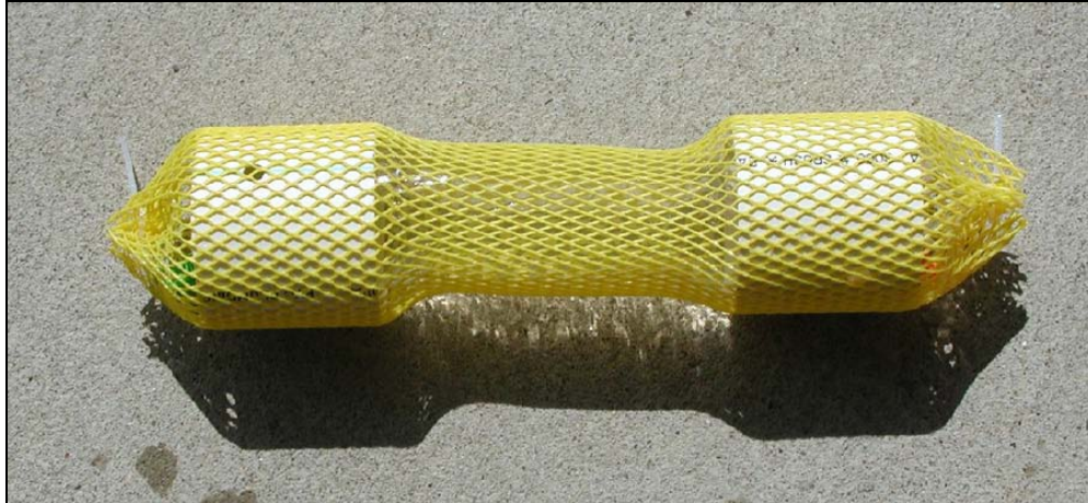
Figure 4. Assembled regenerated cellulose dialysis membrane diffusion sampler with PVC pipe sections external to the membrane.
