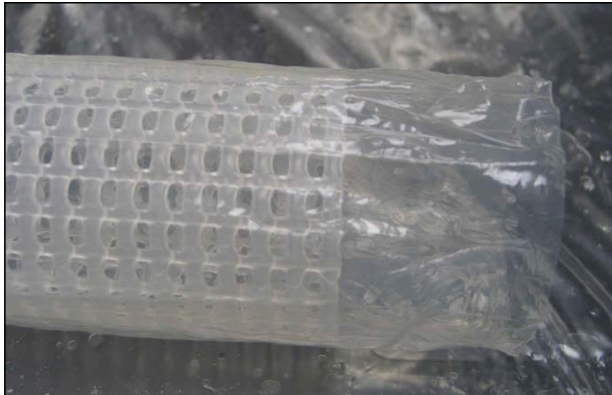
Figure 5. Regenerated cellulose dialysis membrane diffusion sampler with perforated polyethylene support inside the membrane.
