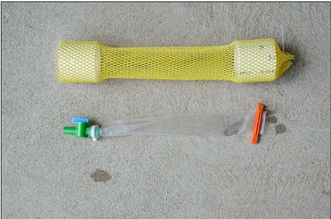
Figure 3. Partially assembled regenerated cellulose dialysis membrane diffusion sampler, showing protective mesh and PVC pipe external to the membrane.
