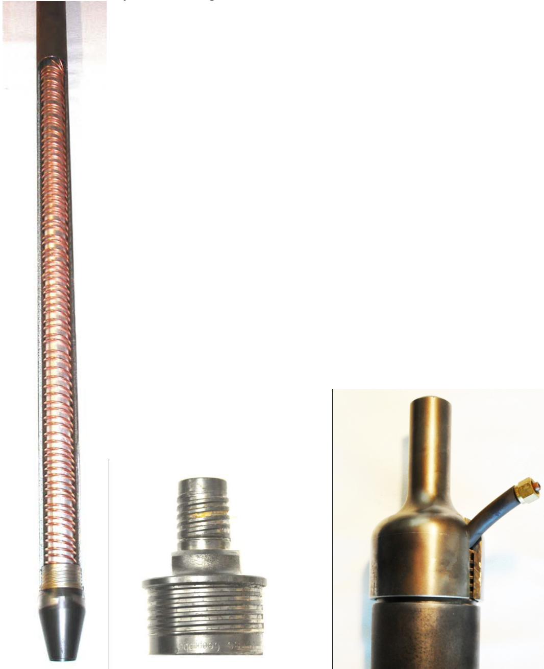
Figure A.1. Prototype Cryogenic Sampler “cut-away” View (left), Adaptor (center), and Slotted Slip Cap (right).
