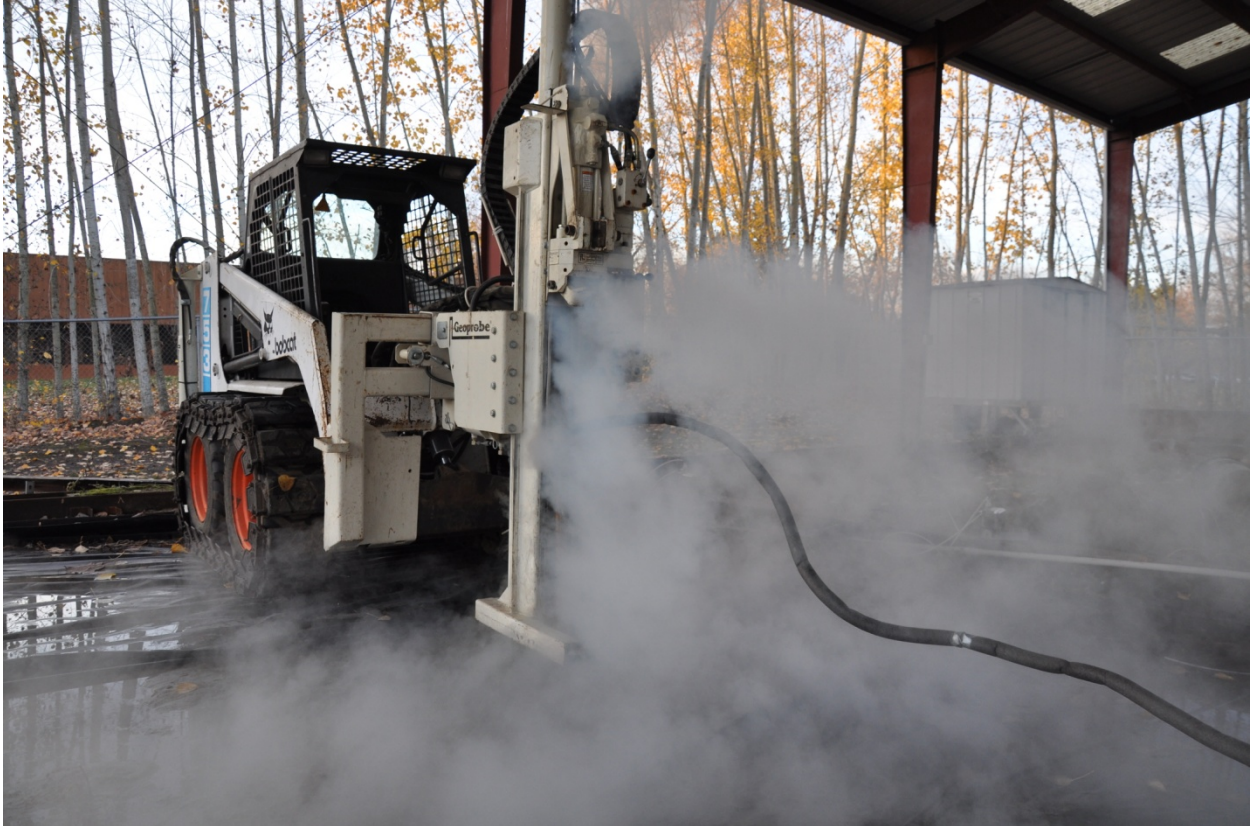
Figure 3.1. Direct-push Cryogenic Coring System Venting N 2 gas During Freezing Phase of Core Collection.
