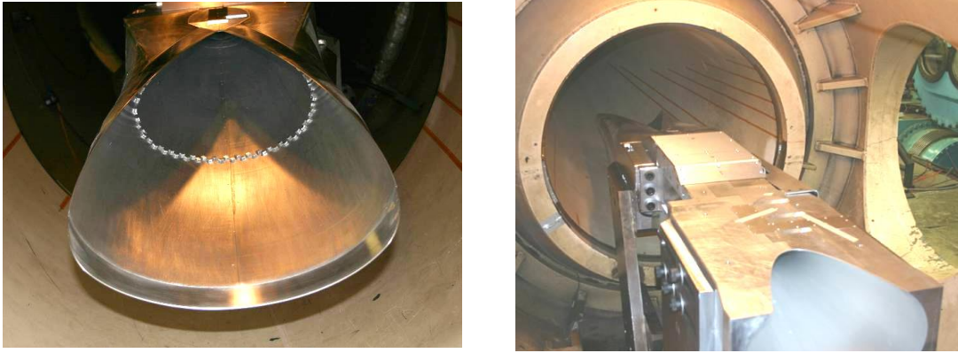
Figure 27: Full-Scale Flight Test Configuration Installed in LENS I Tunnel for Mach 8 Studies
