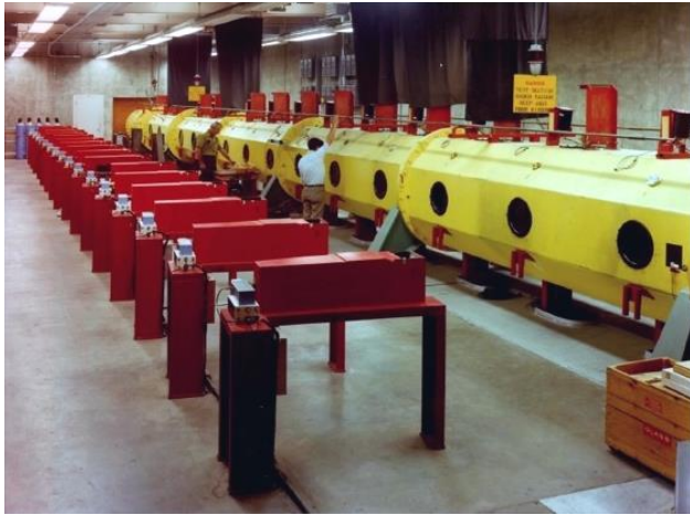
Figure 14: HFFAF test section showing shadowgraph stations.
