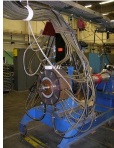
Figure 3: Collector ring assembly.
