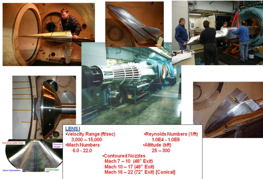
Figure 4: LENS I Reflected Shock Tunnel – Atmospheric Re-entry and Flight for Earth and Planetary Re-entry (Mach 6 to 22)
