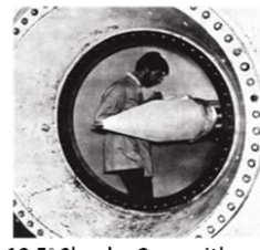
10.5° Slender Cone with Patterned Roughness and Surface Blowing
