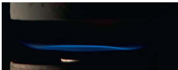
Figure 2: 30-atm helium-diluted flame with helium as shroud gas.
