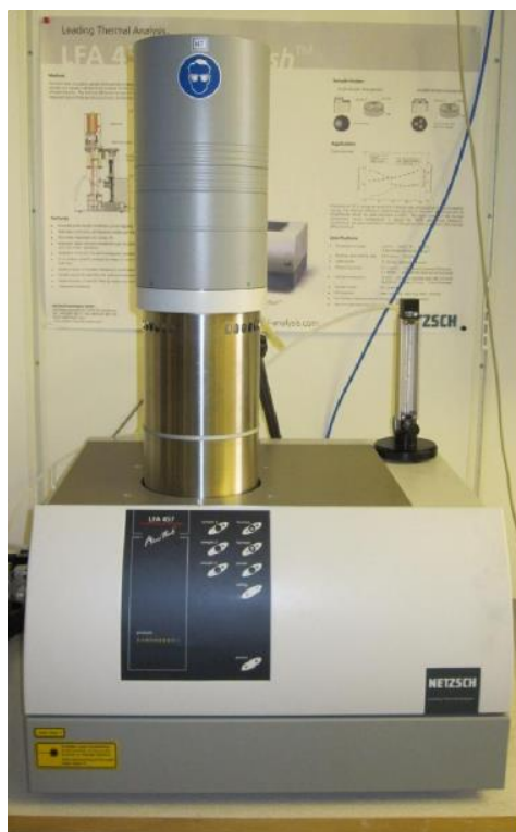
Figure D1: Netzsch LFA 457 Laser Flash Diffusivity Machine.
