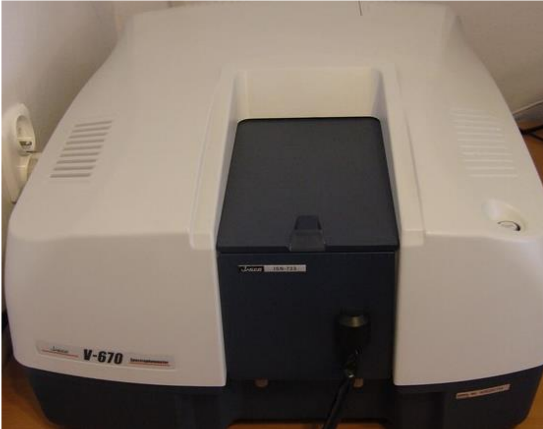
Figure E3: Jasco V-670 NIR/vis Spectrophotometer.
