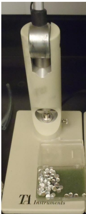
Figure A2: Press used to prepare samples in aluminum pans (shown)
