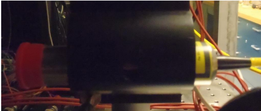
Figure F2: 5.5mm maximum diameter beam collimator
