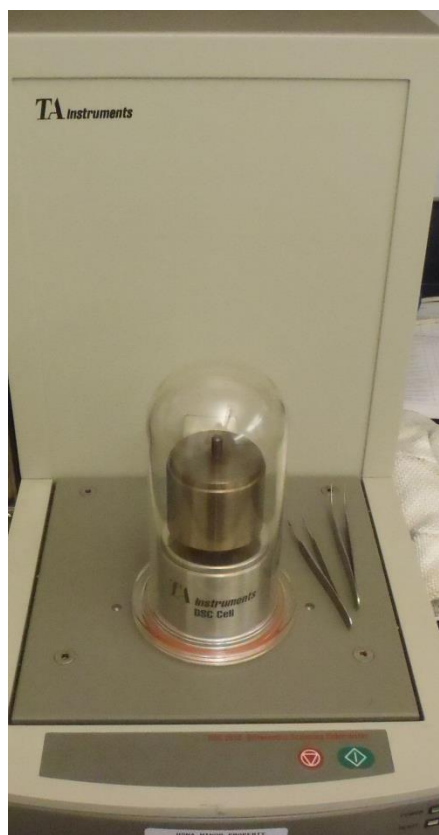
Figure A1: TA Instruments DSC 2010 used for Experiments
