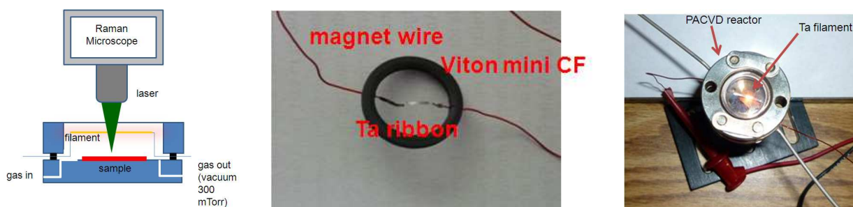
Figure 1: a) Schematic of the modified PACVD reactor b) A Viton gasket modified to hold the hot-wire filament in the PACVD reactor c) Working filament in the reactor cell.
