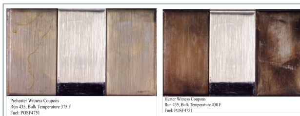
Figure 18. Typical Appearance Preheater/Heater Witness Strip
