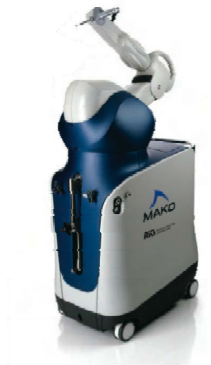
Figure 5.6 The MAKO Tactile Guidance System Assists Surgeons in Minimally Invasive Knee Replacement Surgery
