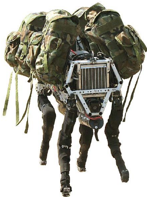
Figure 5.5 Boston Dynamics BigDog Robot Carries Loads for Soldiers
