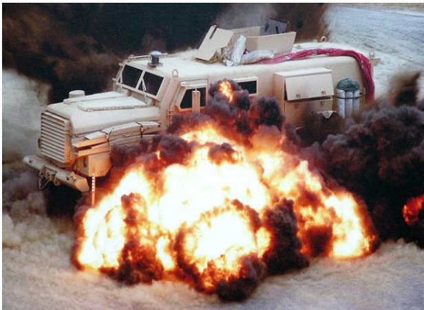
Figure 4a: MRAP vehicle under test.
