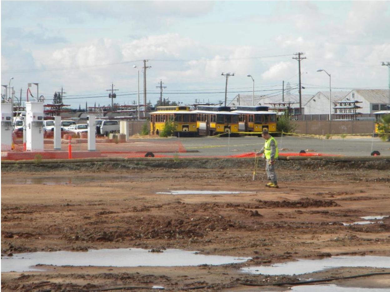
Figure A2-1. Photograph of PRL S-030A, Gamma Walkover Survey
