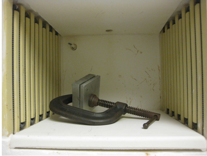
Figure 3.6: Clamp and actuator assembly in oven.
