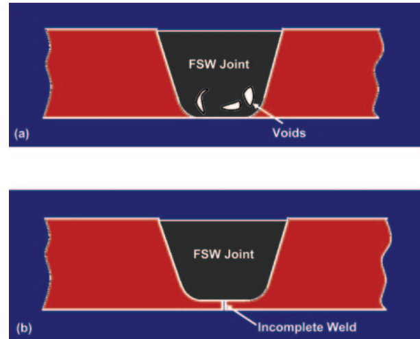
Fig. 6 Two most often observed FSW flaws: (a) voids; (b) incomplete welds
