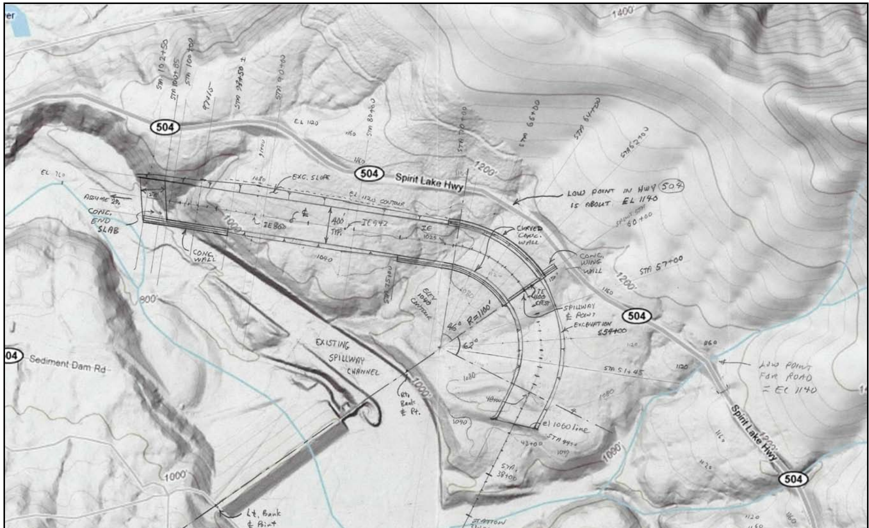
Figure 20. New Spillway Cut in Rock for SRS Raised 160 feet, Configuration 3
