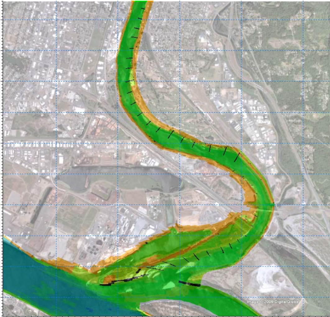
Figure 3. Dikes added to the Lower Cowlitz Model
