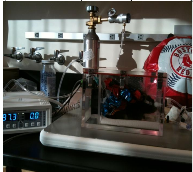
Figure 2: Xenon analyzer, xenon gas supply and recirculation box with connecting tubing and a Mylar reservoir.
