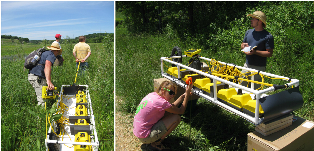
Figure 1: The GPR deployed in tow-mode in Wisconsin (left). Demonstration of free-air calibration procedure we have developed to increase traveltim accuracy.
