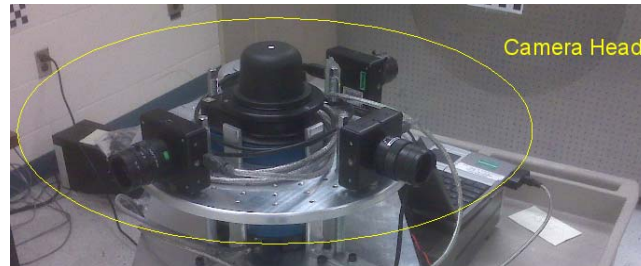
Figure 8: Multi-aperture experimental setup developed by the Alt-Nav team of the Air Force Research Laboratory’s Munitions Directorate; the setup includes three video cameras with a 90-deg separation of their optical axes
